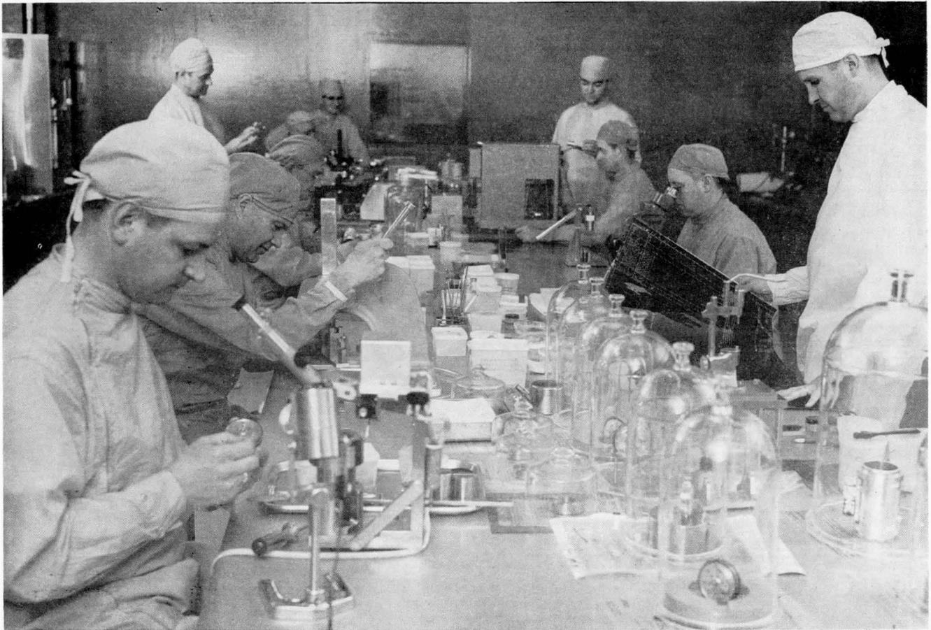
Men at Sperry Gyroscope producing inertial navigation devices under dust-free conditions.
