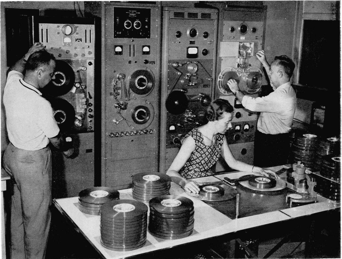
Here, a battery of automatic machines at Audio Devices, Inc., N.Y., makes 100% inspection of magnetic tape intended for use on computers, data processors, instrumentation recorders, etc. Several million pulses are recorded on each reel of tape; if even a single pulse fails to reproduce properly for a tape under test, the machine automatically stops and signals the operator, and the reel is rejected for computer use. (Figure 3)
