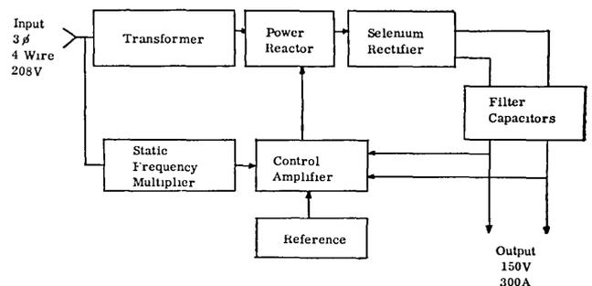
Block Diagram of Magnetic Amplifier System
