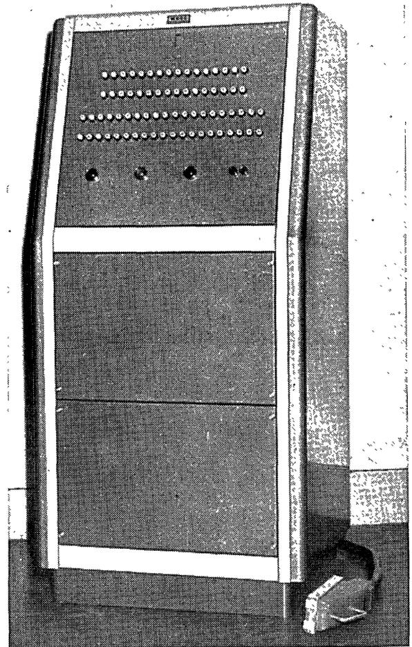
THE WROC 452 IS A SELF CONTAINED UNIT CONTAINING ITS OWN INTEGRAL POWER SUPPLY AND FLEXIBLE CONTROL PANEL DESIGNED TO EXPAND THE CO SELECTOR, PILOT SELECTOR, DIGIT SELECTOR AND EMITTER CAPACITY OF THE IBM 402, 403, 407 AND 408 PRINTING TABULATORS.
