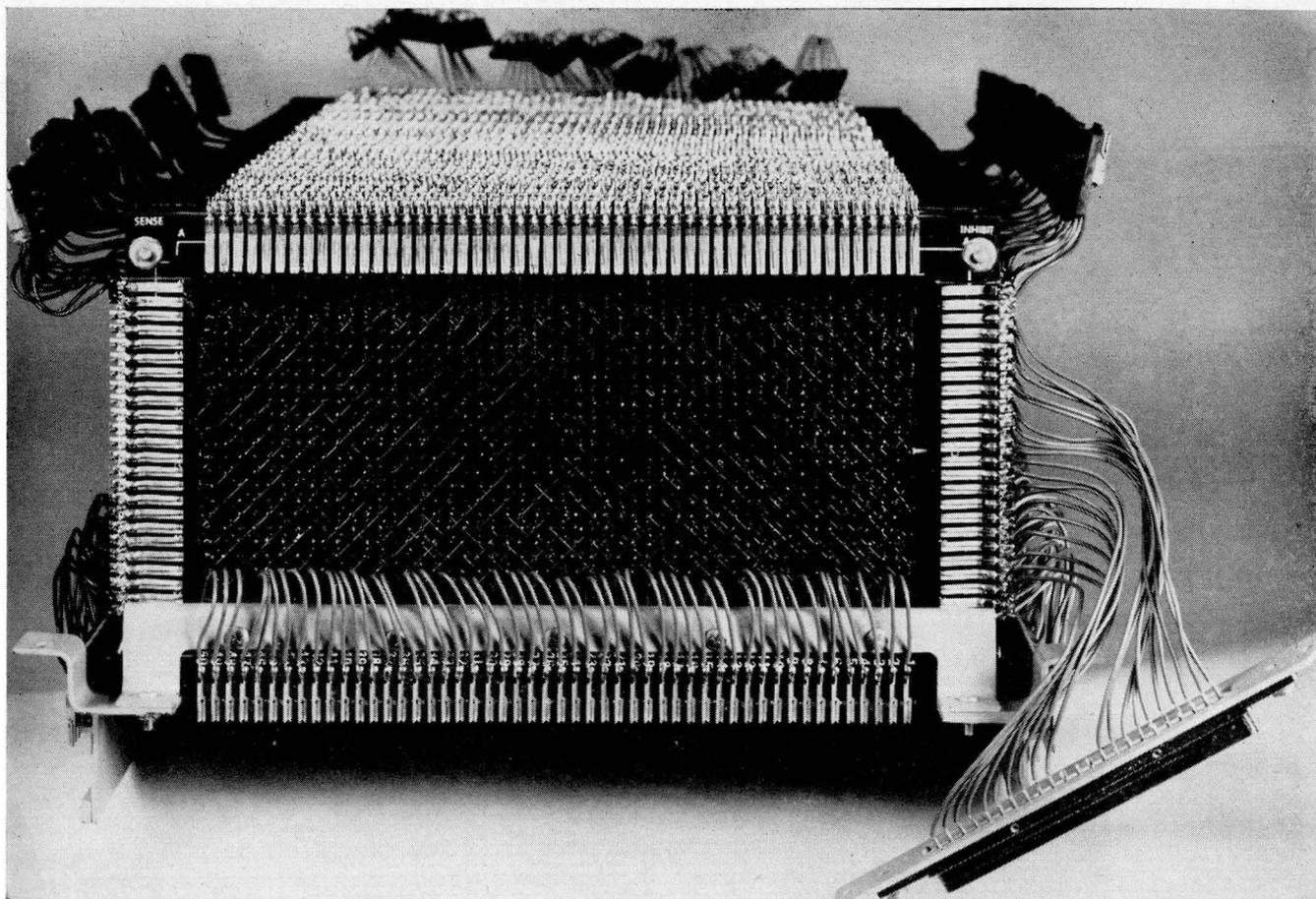
Here is a magnetic core quick-access memory used in a Burroughs 220 computer. In front is the first plane of 1000 tiny doughnut shaped cores. Behind it are 43 more just like it. The memory is entered in parallel by impulsing the same core position in each one of the 44 planes; access time is 10 microseconds. The memory is made by the ElectroData Division of Burroughs Corp., Pasadena, Calif. (Figure 6)
