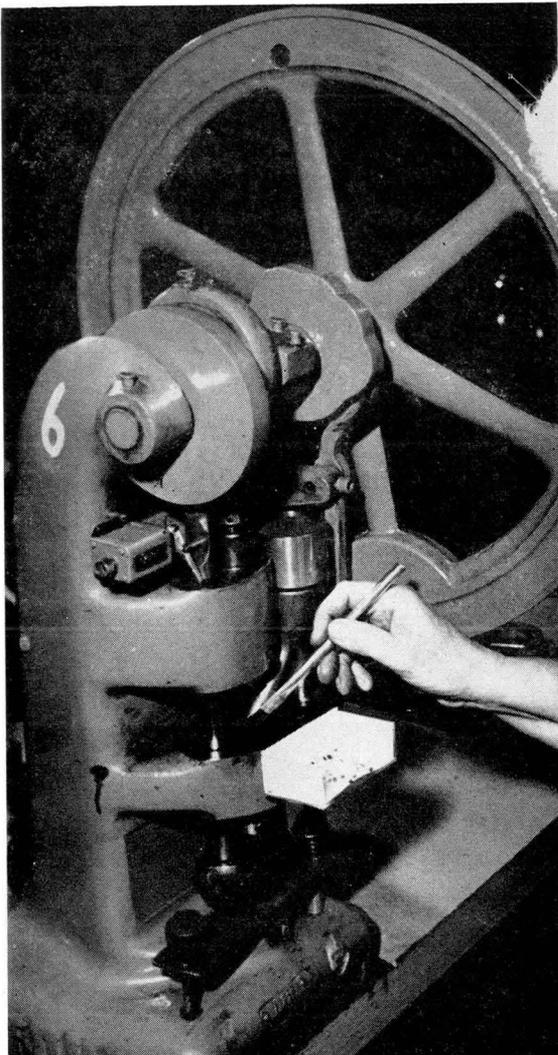
This press squeezes out tiny rings of ferrite powder, which after heating and testing will become ferrite cores for computer memory frames. The place is the RCA plant, Needham Heights, Mass. (Figure 14)
