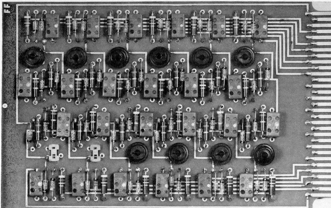
Above is a printed circuit board wired with transistors. It is a plug-in module containing six flip-flop stages. It is used in computers and data processors made by Monroe Calculating Machine Co., Orange, N.J. (Figure 9)
