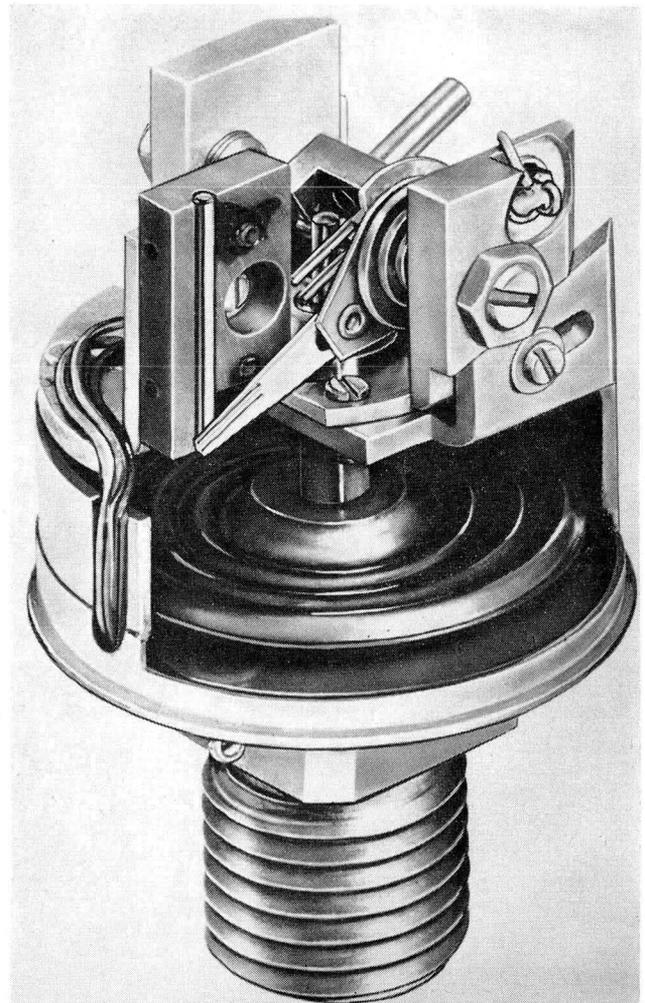
How does a pressure transducer work?—Here is the internal mechanism of a device which senses pressure changes in the range from 0 pounds up to 350 pounds per square inch, and translates the pressure into an electric output using a potentiometer. The movement of the capsule-like diaphragm is converted into the motion of a potentiometer wiper arm. This is a TP-100 made by Fairchild Controls Corp., Components Div., Hicksville, N.Y. (Figure 5)
