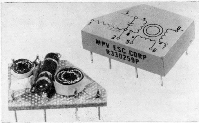
At left is a magnetic shift register, one bit per core, information rate 5000 kilocycle, size 2/10 of a cubic inch, made by ESC Corp., Palisades Park, N.J. (Figure 20)
