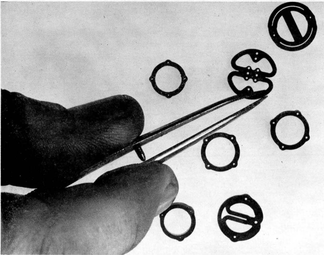
Here are MAD's, or Multi - Aperture Devices, made of ferrite in various forms, and able to perform AND, OR, NOT functions, and other logical functions in computers. They require only single-turn wire for interconnection, are highly reliable, and function over wide temperature ranges. They are still in the experimental stage, being studied at Stanford Research Institute, Menlo Park, Calif. (Figure 18)
