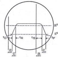
Oscilloscope wave form show typical delay, rise, storage, and fall times achieved with 10-ma inverter circuit utilizing the RCA-2N1301 MESA TRANSISTOR.
