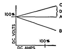
Low-voltage distribution problems can be handled easily through load compensation. Curve "A" is net desired no-load to full-load regulation at load point. "B" is regulation at load without remote sensing or load compensation. "C" represents IR compensation in power supply itself. "D" is amount of IR or load compensation.
