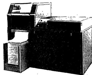
Up to 120 cols. at 600 lines/min. Accepts data from computer buffer or magnetic tape. Vertical and horizontal format control provided.
