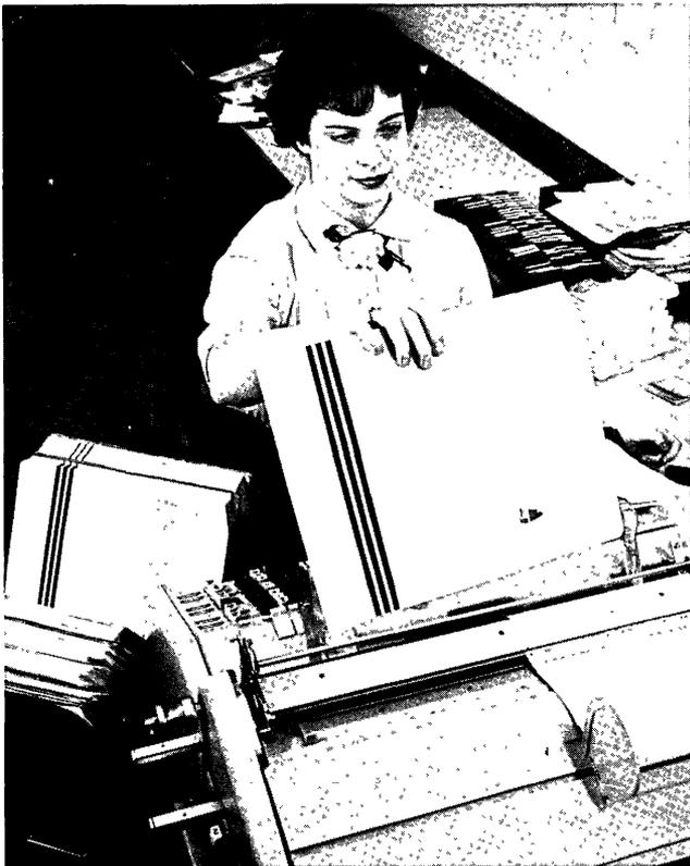
By means of magnetic tracks on the rear of the sheet, recording heads in the machines "read" the new information on the ledger, record the new entries, and automatically update balances -- all within a matter of seconds.
