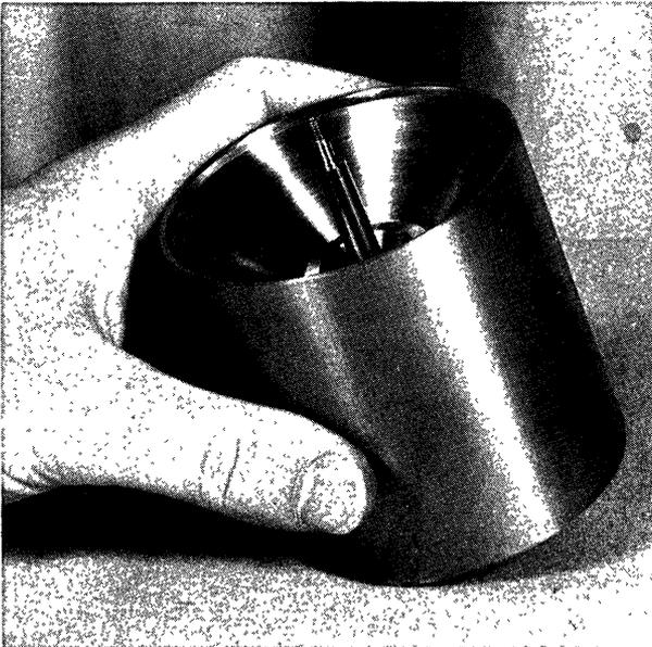
Surrounding the rotating drum is a lightweight frame on which miniature magnetic pickup and recording heads are imbedded in rectangular blocks of plastic called "slider bearings". These bearings slide over the surface of the drum on a cushion of air, staying only 100 millionths of an inch away from the drum even under the most severe vibration conditions.
