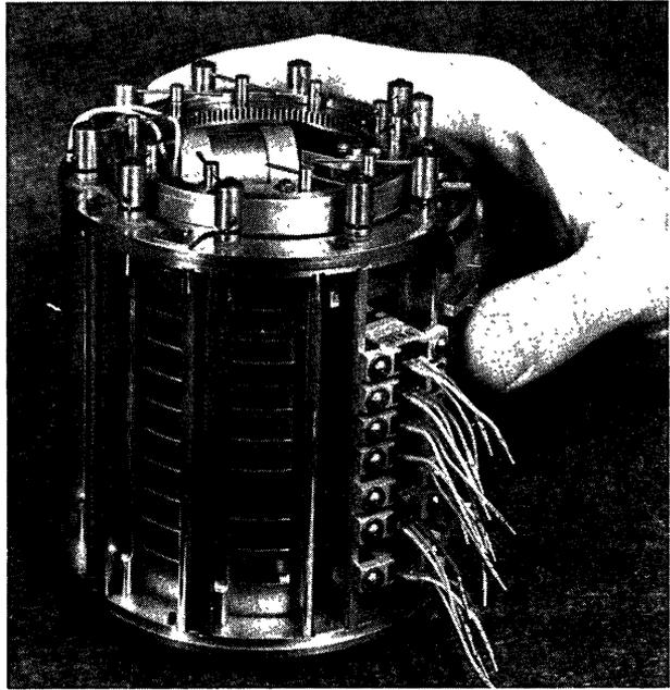
Total weight of the miniature drum assembly is 8 pounds, compared to about 235 pounds for conventional drum assemblies.
