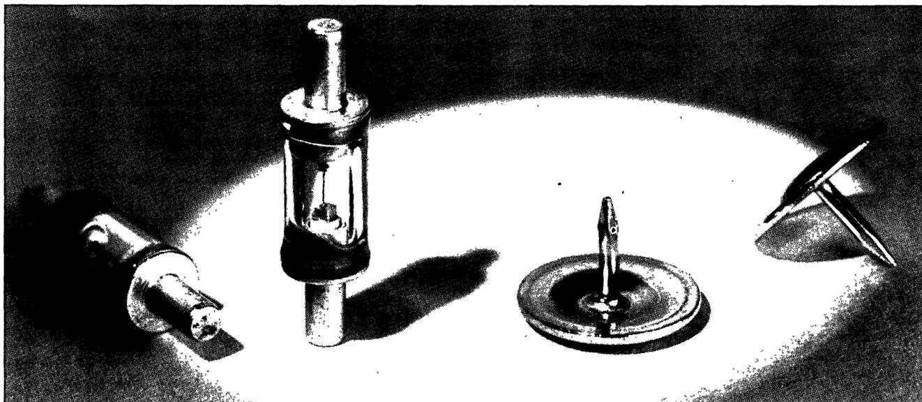
This company has introduced the first microwave crystal diode designed to switch power up to 100 milliwatts at speeds of less than one nanosecond (one billionth of a second) -- the 1N3093. The picture shows it compared with ordinary thumbtacks.
