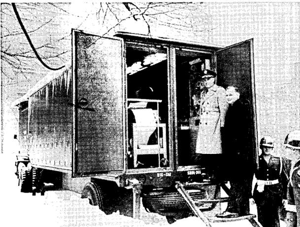
MOBIDIC is made rugged for movement and operation under extreme environmental conditions. Emphasis in design was on performance with extreme reliability in combat, and resistance to extremes of shock, vibration, humidity, dust and temperature. In the hard road testing of ruggedization at the Aberdeen Proving Ground, the truck containing the computer developed defects and not the computer.
