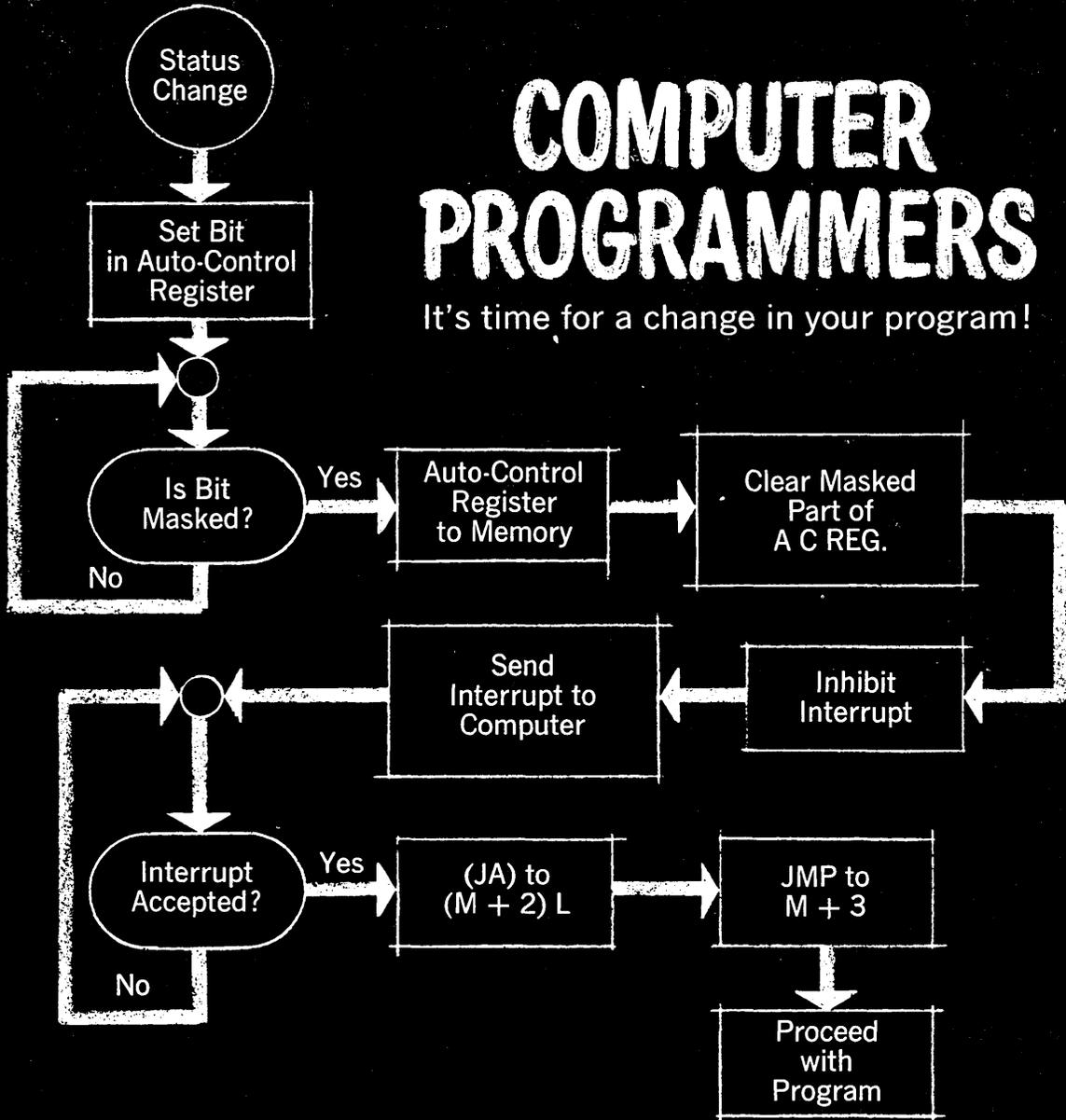
The Auto-Control Unit of the PHILCO 2000 provides a means of interrupting a program whenever specified conditions appear . . .
