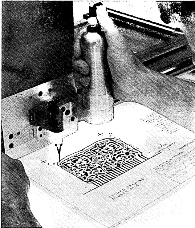
The new automatic equipment consists of two units, each of which can be operated independently. The first device is a drawing-to-tape converter which generates a completely programmed one-inch-wide eight-channel punched tape directly from a dimensionless drawing outlined on a 1/10 inch grid pattern. The
