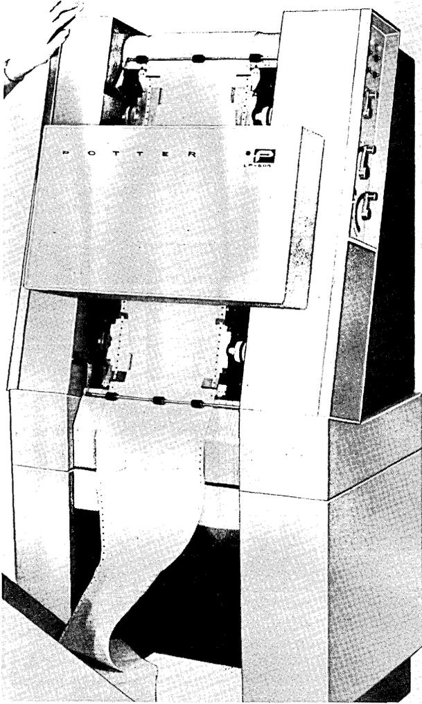
carriage, and a static-electricity paper discharger at the output end of the printer. The paper-feed system eliminates form skewing. Modular solid-state electronics are used throughout the printer. At the Eastern Joint Computer Conference in Washington in December, it operated continuously throughout the show without down-time or adjustment.
