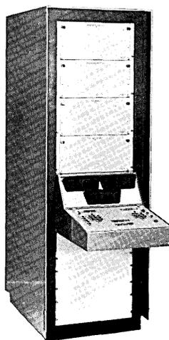
**CI-70 Precision Potentiometer Positioning System** provides fully automatic tape or card set-up for coefficient potentiometers, diode function generators and UNE's. Programming time is reduced by a factor of 5. Potentiometers are set in less than 2 seconds each, with error no more than 10 millivolts. Other features are automatic scan, automatic check-out, and automatic error indication.
