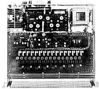
An interior view from the top shows the magnetic core storage array (upper right hand corner) and universal printed circuit boards containing core driving and sensing circuits. The complete memory is packaged in a standard 19 inch relay rack 3 1/2 inches high and 16 inches long.
