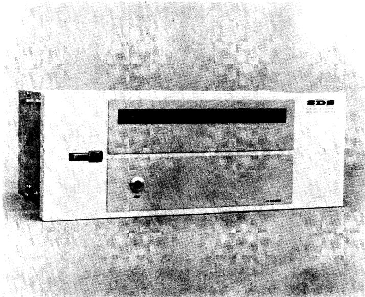
AD Series of analog to digital converters -- Scientific Data Systems, Inc., Santa Monica, Calif. / The AD Series of analog to digital converters are high-speed, all silicon semiconductor devices that operate at speeds in excess of 5 microseconds per bit. They operate from 0° to 100°C. Transformer coupling is provided for all digital control and output signals in order to eliminate system grounding problems.
