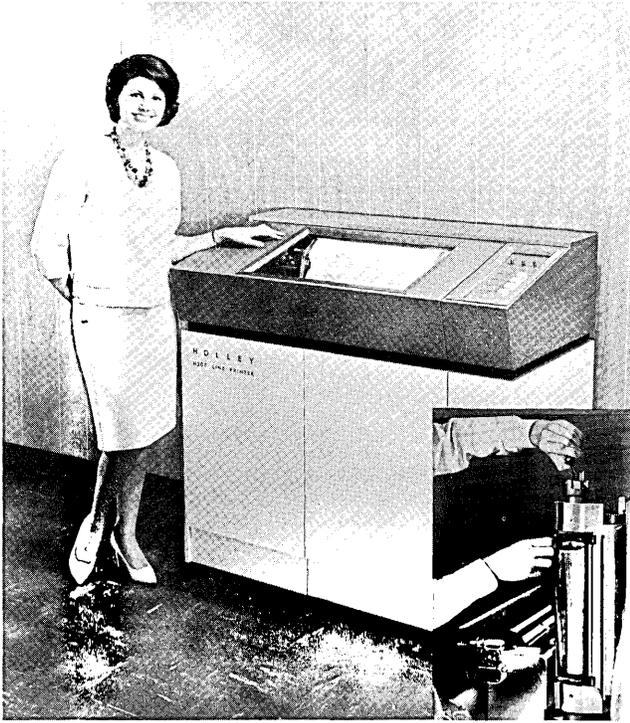
A new model of the H207 medium-speed line printer has a print ribbon claimed to have three times former life. When 64 characters are printed, line speed is 300 lines per minute. Interchangeable print drums (see photo insert) allow increased speed when a large selection of characters is not needed. A swing-up drum arm permits easy forms loading. A printer control, cabinet, and buffer for character serial input are optional with the print head.
