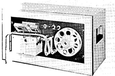
The Facitape Model 110 reader (shown above) has a capacitance read head, which is unaffected by ambient light conditions, dust or lint on the read heads, or other environmental hazards. Speeds up to 600 characters per second are obtained and the reader will stop within one character through its entire operating range. All 5 through 8 channel tapes may be read in any desired code.
