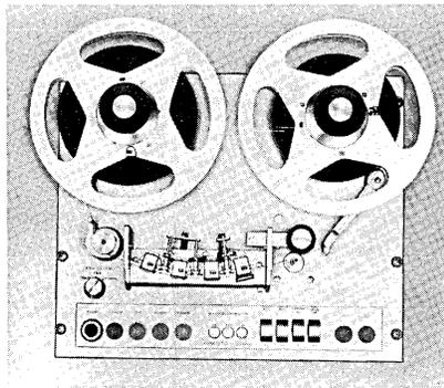
The transports have a four-head plug-in assembly; seven tape speeds ranging from 15/16 to 60 inches per second; selectable tape width; separate cue and edit controls; balanced braking; illuminated "feather touch" controls; and remote control on all modes. Available heads with 1/2 inch tape can record up to 14 different phenomena simultaneously.
