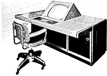
A new technique in solid-state character generation enables formation of up to 500,000 characters per second. Each is composed of from one to 25 individual line segments.
