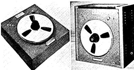
The Model K-80 accomplishes erasure by rotating the tape reel through a gradually-reduced, high-flux density alternating magnetic field employing three separate magnet coils. Erasure level is 80 to 95 decibels, depending on the method of measurement.
