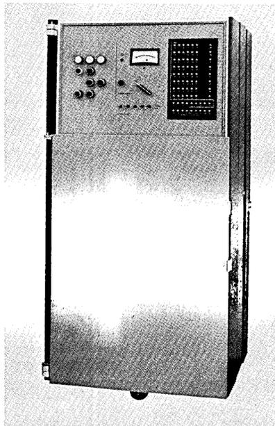
The LZ has a storage capacity of 4096 to 16,384 words with word lengths of 18 to 72 bits. Operational modes are read-restore and clear-write. Control signals are read-request and write-request. Along with its complete cycle time of 1 microsecond, its read access is 0.5 microseconds after read request.
