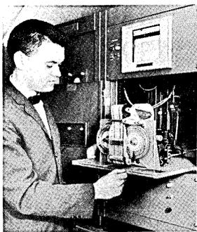
— Walter E. Jackson, shown checking the ADR which records the nitric oxide present in the air, is in charge of the Philadelphia station. On the right is a section of the punched tape record that each ADR instrument supplies for a specific air pollutant.
