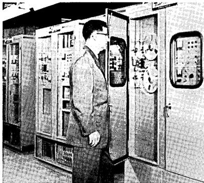
above, will operate a 3-axis Pratt & Whitney Numeric Keller machine at Boeing.
