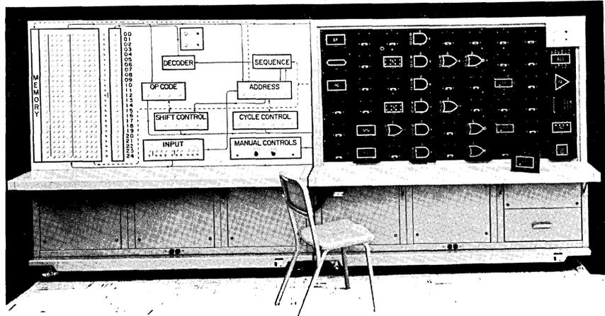
The 6B4 consists of two training demonstrators combined in a single unit: a realistic small-scale digital computer; and a flexible logic demonstrator. As a Digital Computer Trainer, the operation of a small-scale general-purpose computer is displayed on the twelve-foot face of the system in flow diagram form. The contents of the special twenty-five word memory, as well as all major
