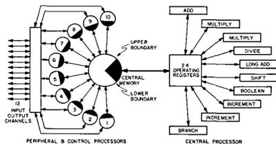
Fig. A -- Block Diagram of 6600
