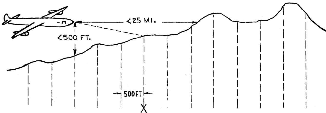
Figure 4. Terrain Avoidance Guidance
