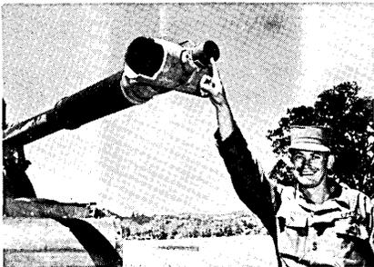
— The "killing" end of the Hit-Kill Indicator is a photo-electric telescope in the tank's barrel which exchanges infrared signal pulses with the target to make the "kill". The photo-electric device, which completes a "fire mission" in less than a half second, can be used for weapons capable of 4000 meter ranges, while other versions are man-portable for simulated combat with the M-14 Rifle.
