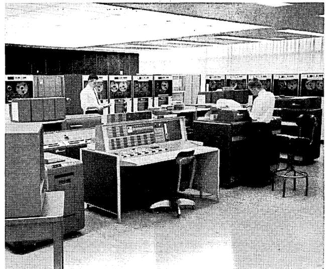
An IBM 7094 in M.I.T.'s Computation Center can be operated from the classroom via a time-shared console.
