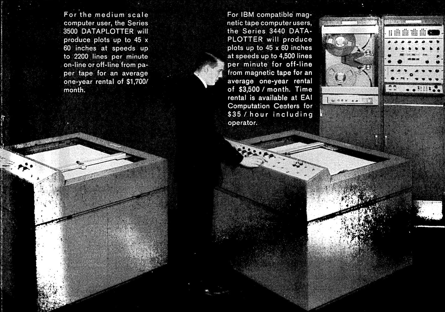
For the medium scale computer user, the Series 3500 DATAPLOTTER will produce plots up to 45 x 60 inches at speeds up to 2200 lines per minute on-line or off-line from paper tape for an average one-year rental of \$1,700/month.
