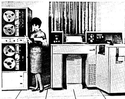
— UNIVAC 1004 III Magnetic Tape System can be used as an independent data processor, a satellite system for large-scale computers, or operate on-line with the UNIVAC 1107 or the 490 computers.
