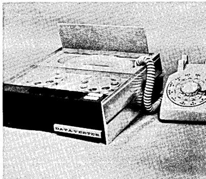
— The Data-Verter system transmits data over telephone lines. Data is entered into the recorder on magnetic tape and in machine language. The tape cartridge is then inserted into the transmitter (shown above) and is sent over telephone lines to the remote computer, at speeds up to 500 words per minute.
