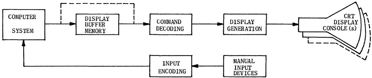
Figure 1a. The general purpose console display.
