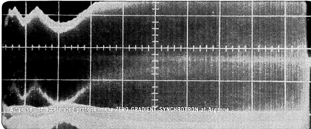
A "pulse" of accelerated protons in the ZERO GRADIENT SYNCHROTRON at Argonne.
