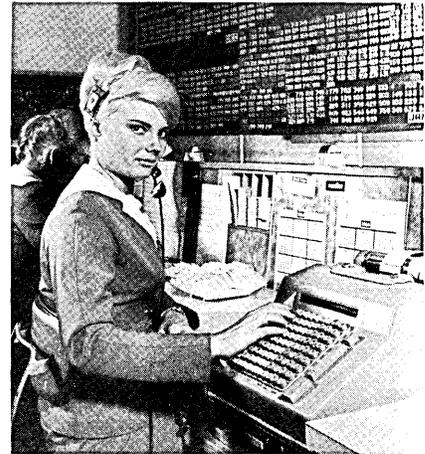
on special NCR inquiry machines which are directly connected to the NCR 315 computer in an adjacent room. In less than a second the computer checks seating space for any flight and indicates by signal light on the operator's machine "OK" or "Flight Booked". (PSA's 35 outlying ticket agents are linked via a private telephone network to the reservations center.)
