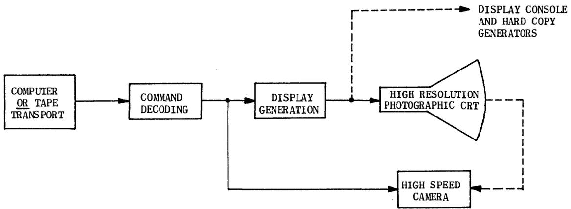
Figure 1b. The high speed film recorder.
