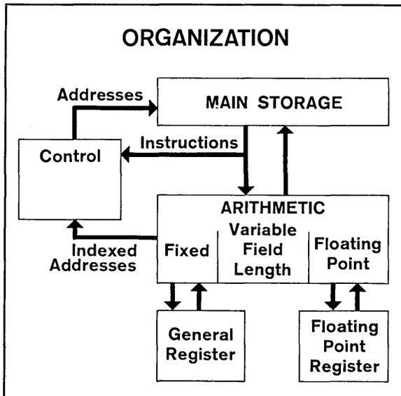
Figure 1 shows the organization of all processing units available with the System/360. Each processor has a main memory; a local store in which index and address registers and arithmetic results are kept; an arithmetic section where additions and comparisons are actually done; and a control section which, in all but one processor, uses read-only storage to tell the arithmetic unit how to accomplish a desired task.
