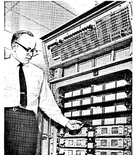
— UNIVAC CP-667 military computer. The thin film memory can be tested by a flip of a margin switch, shown here by a UNIVAC design engineer. The upper four roll-out chassis contain semi-conductor integrated circuits. The remaining eight chassis house the main memory of almost five million cores.
