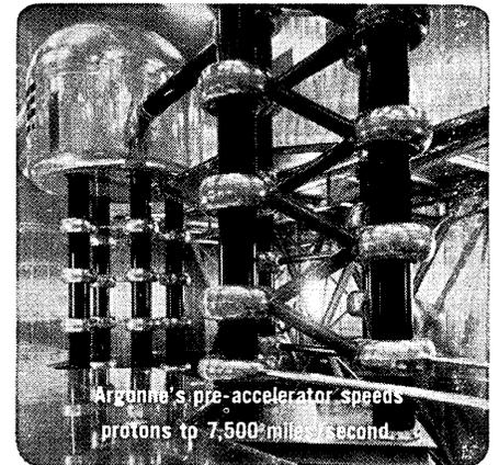
Argonne's pre-accelerator speeds protons to 7,500 miles per second.
