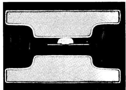
— Double-sealed glass diode. This diffused-junction epitaxial diode, called the Microglass diode, attains design flexibility by adding any type of lead for direct replacement of current diode types.
