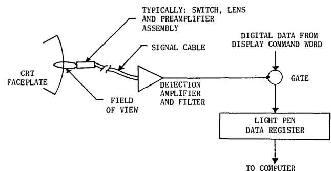
Figure 4. Functional arrangement of a light pen.
