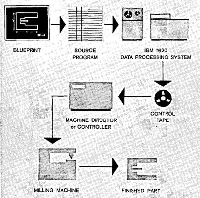
The chart above illustrates how a small-scale data processing system, the IBM 1620, can help produce a finished part from a blueprint drawing. The computer, operating under control of the new program AD-APT, converts English-like statements from a source document into instructions for numerically controlled machine tools. These instructions then direct the machine tool through the cutting operations necessary to produce the finished part called for in the blueprint.
