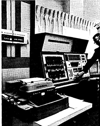
— New low-cost hybrid analog/digital computing system shown consists of Packard Bell's PB250 digital computer (left) and T-50 desktop analog computer manufactured by Compu-ter Products, Inc.
