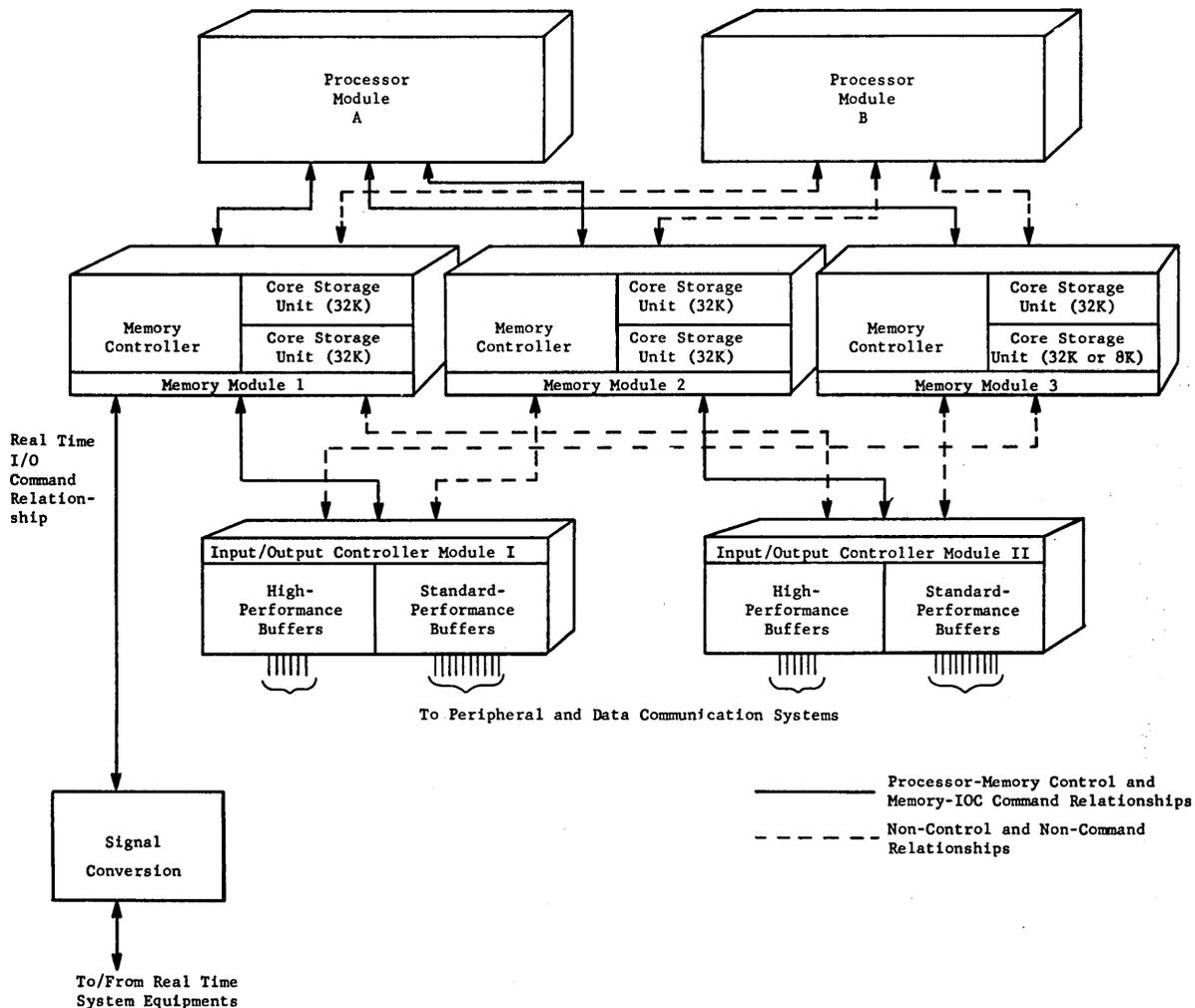
Figure 1. Typical Multiprocessor Configuration of a GE-600 Computer With Real-time Capability
