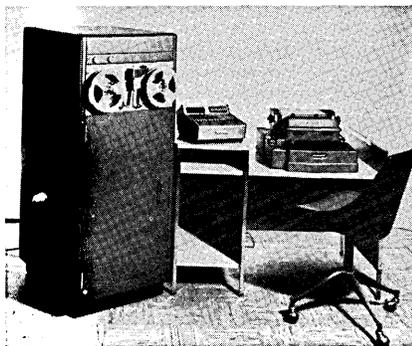
The machine is compatible with any input-output keyboard or tape typewriter chosen by the user. It will accept and produce 5, 6, 7, or 8 channel tape up to 1 inch wide, in any tape code. Tapes are processed at rates of 500 words per minute.
