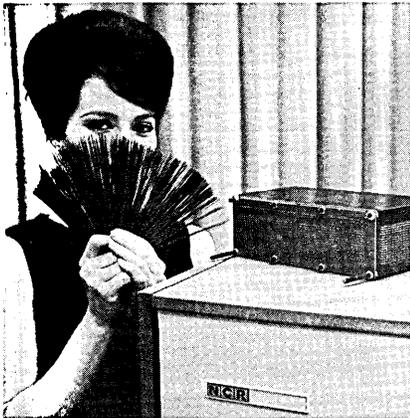
— Miss Marie Coates of NCR's Electronics Div. displays some of the thin-film Rods used in the 315 RMC. A memory module is shown on top of the cabinet.
