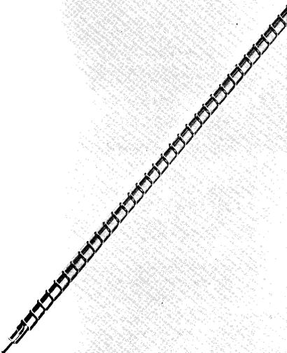
— Microscopic view of one of the Rod elements used in NCR's new 315 RMC (Rod Memory Computer).
