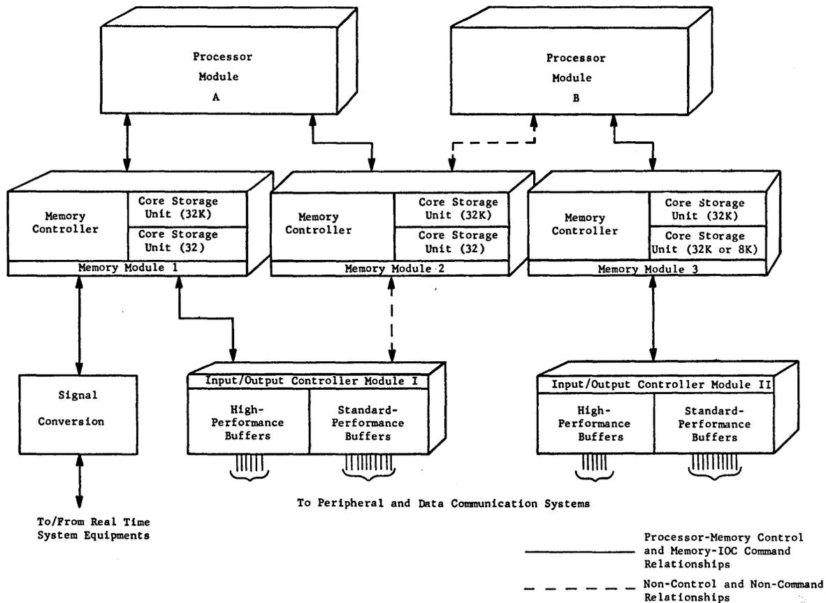
Figure 2. Typical Multicomputer Configuration of a GE-600 Computer
