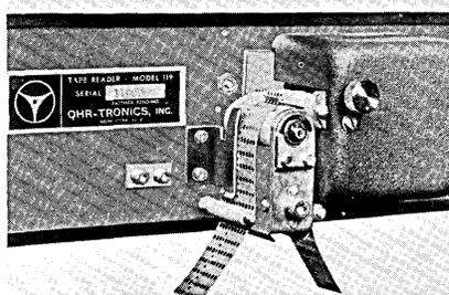
A twelve point commutator is mounted on the sprocket shaft. All points are brought to a 36 pin connector with mating connector supplied. Standard units are wired for 24, 48 or 90 VCD. Coils are designed for continuous duty and are arc suppressed with diodes. Interrupter switches are provided for self-stepping and electrical interlocking. (For more information, circle 53 on the Readers Service Card.)
