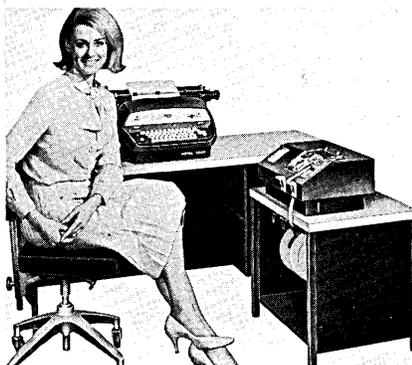
The Royal 5000 SDW can be operated from the keyboard at speeds of up to 25 characters per second. Tape can be regenerated at speeds of up to 50 characters per second.
