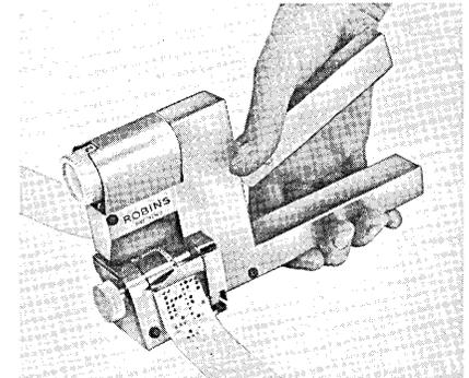
A selector knob in the front of the device permits quick and easy selection of the code desired. An indicator window at the top front shows the exact character being punched. After each code is made, the tape is automatically fed to the next punching position. (For more information, circle 54 on the Readers Service Card.)
