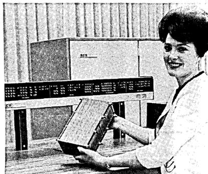
— NCR's new 315 RMC (Rod Memory Computer). Miss Marie Coates of NCR's Electronics Div. holds a section of the new memory which contains wire Rods coated with magnetic thin film.
