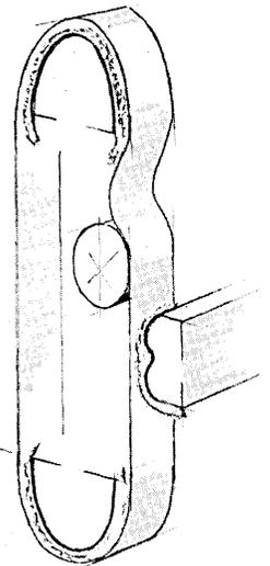
tape loops float over stationary bearings on cushions of air... "fly" past write/read head without making physical contact. Years of trouble-free operation are assured.
