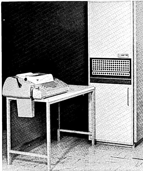
DDP-116 / Computer Control Company, Inc. — This low cost, 16-bit digital computer has indexing, multi-level indirect addressing and priority interrupt. It performs up to 294,000 computations per second. Basic memory cycle is 1.7 microseconds; add time is 3.4 microseconds; and the memory is expandable up to 32,768 words. The DDP-116 is designed for both open-shop scientific applications and real-time data processing. (For more information, circle 49 on the Readers Service Card.)
