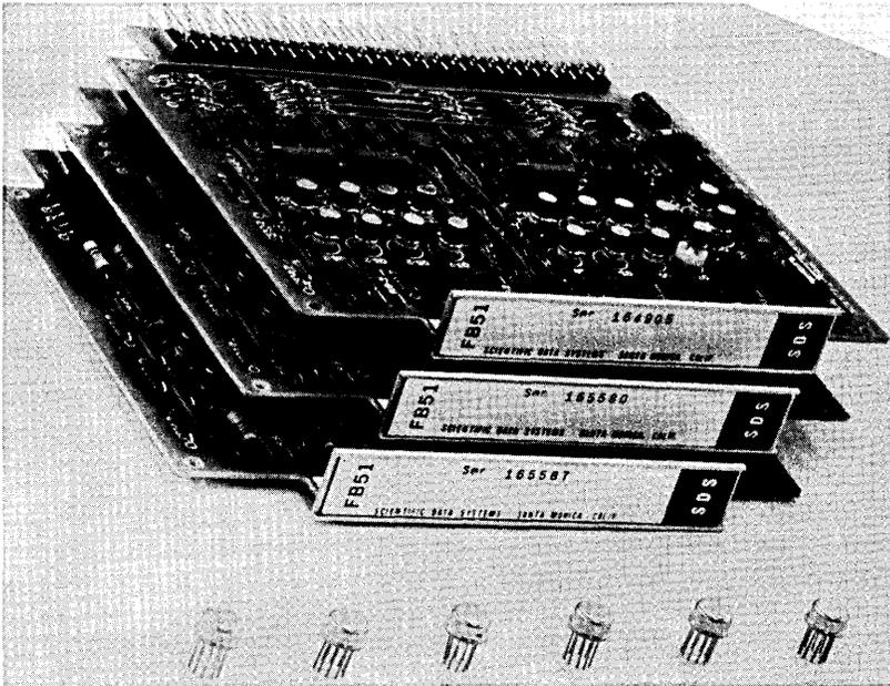
**INTEGRATED CIRCUITS** / Scientific Data Systems, Inc. — The six little cans with leads (shown at the bottom of this picture) are integrated-circuit flip-flops, which, along with other related components, are mounted on a single printed circuit card in the new SDS 92 computer. They are the equivalent of the three printed-circuit cards (shown at the top of the picture) if conventional circuit elements were used. (For more information, circle 104 on the Readers Service Card.)
