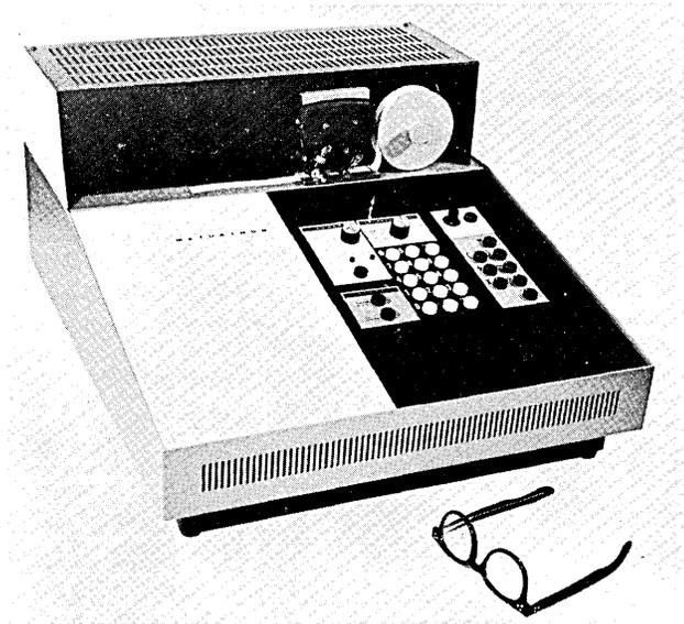
MATHATRON / Mathatronics, Inc. — This desk-top computer/calculator includes a ten-key direct input keyboard, storage registers, ferrite-core program memory storage, solid-state computer logic, and printed output. Extra storage registers, program memory storage, constants and special pre-wired programs may be added to suit individual computing needs. (For more information, circle 53 on the Readers Service Card.)
