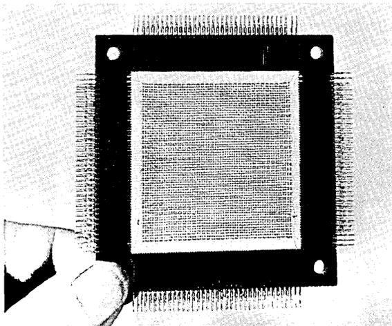
20 MIL FERRITE CORES / Ferroxcube Corporation of America — To meet the increasing demand of high speed memory systems, ferrite core planes and stacks are being produced which make 1 microsecond cycle times for coincident current memory systems possible. These new devices have 20 mil diameter cores with 180 nano-second switching times. They are available in various bit and winding configurations. (For more information, circle 107 on the Readers Service Card.)
