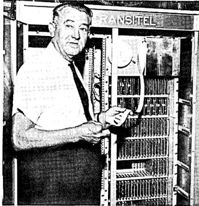
— Transitel meter data receiver. Mr. Leo Duffy of the Consumers Power Company holds 8-level punched paper tape on which the readings are recorded.
