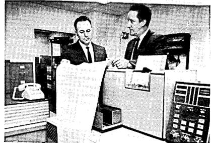
— After calling the firm's computer center, using the Bell System Data-Phone data set at left (top), a clerk inserts punched cards into a Honeywell transmission unit for relay over phone lines directly to the computer which runs a credit check on them. Within hours the originating office receives back information (bottom) on persons identified as having a record of credit delinquency.
