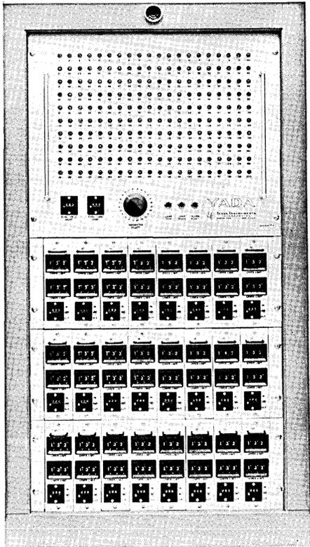
YADA, MODEL 858 / Texas Instruments, Inc. — Yield and Distribution Analyzer (YADA) Model 858 for punched card data analyzing quickly summarizes data which pass within preset limits compared against preset upper and lower values. A yield counter totals the units passing; a device counter totals units compared. The 858 analyzes three or four digit parameters and will read and compare 72 columns of an 80 column IBM card simultaneously. (For more information, circle 62 on the Readers Service Card.)
