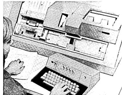
**IBM 29 CARD PUNCH** / IBM Corporation — The IBM 29 card punch (shown in photo) and its companion, the IBM 59 card verifier, are used to record and check information in cards. Cards then are read and processed by a computer or an accounting machine. The new devices can store two different punching formats as a standard feature. Both devices have 64-character sets (a 48-character set also is available). (For more information, circle 92 on the Readers Service Card.)
