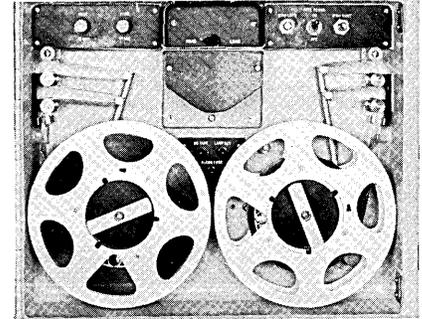
**500RM TAPE READER** / Photocircuits Corporation — The reader utilizes a printed motor direct capstan drive for tape transport, completely eliminating pinch rollers, brakes and clutches. The 500RM will read at speeds up to 500 characters per second and will Wind/Search at 1000 characters per second. The device will accommodate 5, 6, 7 or 8 level tape and has 8 inch reels. Optional polarities for input and output are available. (For more information, circle 98 on the Readers Service Card.)
