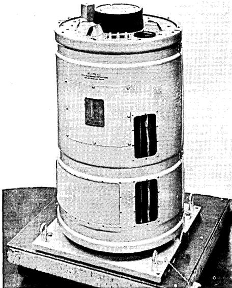
TYPE 371-14 MAGNETIC MEMORY DRUM / Ferranti Electronics Division of Ferranti-Packard Electric Ltd. — The 371-14 magnetic memory drum is capable of storing up to 6.4 million bits at 425 bits per inch on 480 tracks. Error rates are less than 1 in  $10^{11}$  bits transferred. The complete drum system consists of the drum, drum controls, read amplifiers, write amplifiers, track selection circuitry and power supplies. (For more information, circle 86 on the Readers Service Card.)
