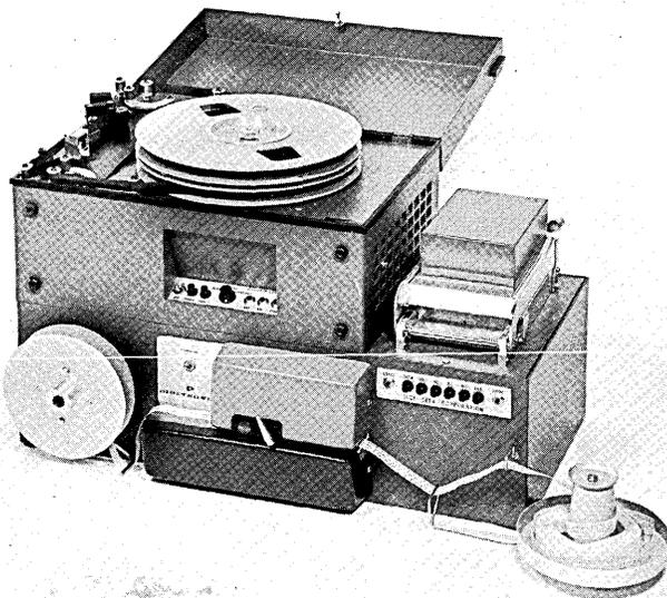
**MODEL 1720 PAPER TAPE TO MAGNETIC TAPE CONVERTER** / Digi-Data Corporation — This unusually small device has a high reliability rate coupled with ease of service. Its' broad programming capabilities are by means of a plugboard. Use of this system makes a typewriter or add punch into an effective computer entry device. (For more information, circle 66 on the Readers Service Card.)
