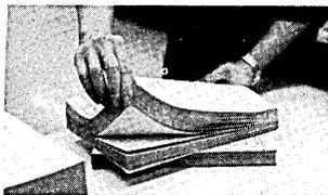
The finished stack is then taken to a padding station (photo, upper right) where a special penetrating adhesive is applied and the forms are allowed to dry. Then the padded stack is fanned apart (bottom) into unit sets with the simple flick of a thumb down the side of the padded stack. Forms are produced with the pre-collated paper in half the time it takes to make carbon-interleaved forms for approximately the same cost. (For more information, designate #41 on the Readers Service Card.)
