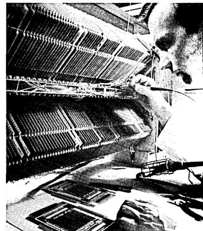
lated selection wires into a high-density mesh. The intersections of the wires form bits that store large amounts of information in extremely small areas.
