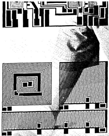
Glass plates were chosen for their transparency and dimensional stability. High strength is required to reduce loss of the costly circuit masters and to protect personnel and equipment.
