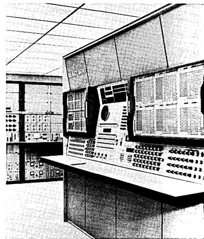
The standard model of the REAC-600 contains 300 solid state operational amplifiers of a new high speed type, giving it many times the problem-solving capacity of previous REAC models. End uses of the REAC-600 include design of space, automotive and other systems, automated railroad switching and many types of industrial and scientific research. (For more information, designate #44 on the Readers Service Card.)
