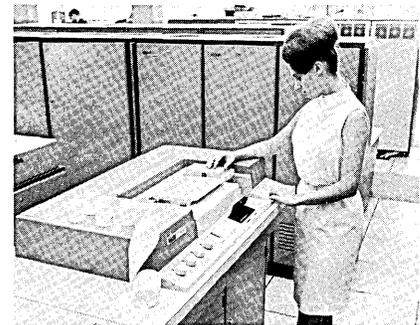
isters, adding machines and accounting machines equipped with optical typefonts, the company reports. The 420-2 reader scans 52 lines of print per second at up to 32 characters per line for a maximum of 1664 characters per second. This reader is internally programmable and has fast (10-second) tape change, automatic editing and variable output formats.
