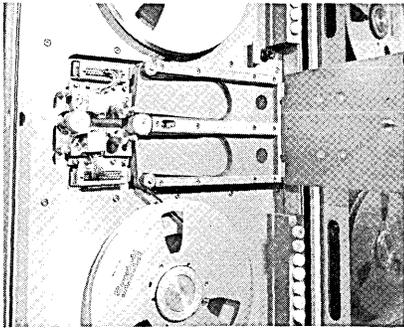
— Honeywell 7600 transport deck with dual vacuum column doors open shows simplified, bi-directional tape drive unit of the new tape system
