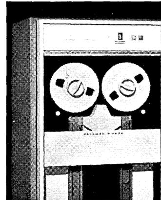
The **D 3030** writes and reads all three densities (800, 556 and 200 cpi) at 75 ips tape speed. Push-button selection of 60,000, 41,700 and 15,000 cps data transfer rates. Either 7-track or 9-track format. Vacuum column tape buffers, semi-automatic tape threading, front access to all electronics, and many other advanced features. Bi-directional start and stop times of 5 ms and 1 1/2 ms, respectively.
