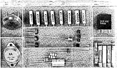
— Unique spare parts kit includes selection of micrologic circuitry, transistors, diodes, trim pots, pilot lamps and fuses, plus a relay, an inductor, and a capacitor
