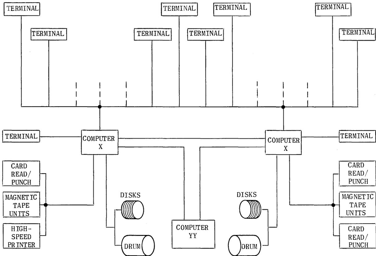
Fig. 1. One Configuration for a Computing Utility Central
