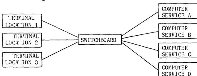
Figure 2. Terminal Switching Network.
