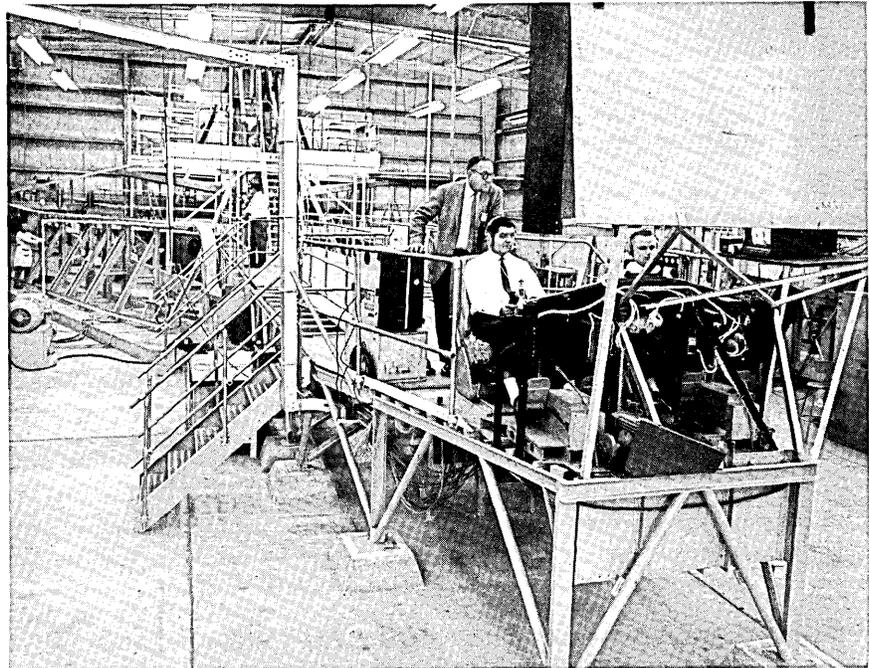
— Boeing Company engineers "fly" the firm's 737 Iron Bird, first used in the development of the Boeing 727 trijet and completely redesigned and rebuilt for the 737. Technicians in the background check the action of the ailerons.
