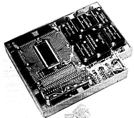
It uses only 1.25 watts of power — less than the amount used to turn on a flashlight — to transfer data at a rate of 5000 pieces of information a second. All information is stored in 128 memory words which are randomly accessed. Each word is 21 bits long and is read out a bit at a time.
