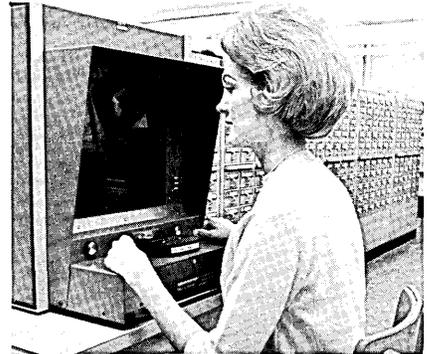
— Betty Woodall uses a microfilm reading machine in Lockheed's technical library to scan a microfilm roll of authors. Information encased in 720 card files like those in background have been processed by a computer system and compressed into 40 microfilm cartridges.
