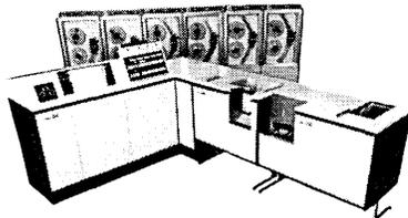
The Univac® 9300 is the second unit in a series of interlinking computers. (You know: you start with any one, and simply build on it as your computer needs grow.) The Univac 9300 brings you from punched cards to magnetic tape data processing in one small inexpensive step. It's the first high-speed tape system the small computer user can afford.
