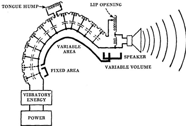
World's Fair in 1939. The Voder used two electrically-generated complex vibrations to create the sounds, a buzz representing the larynx tone (voiced sounds) and a hiss consisting of random noise (unvoiced sounds). Either of these sounds was applied to a group of bandpass filters which covered the range of speech frequencies. Each filter was separately controlled, and the outputs were combined, amplified and applied to a loudspeaker to form synthetic speech sounds.
