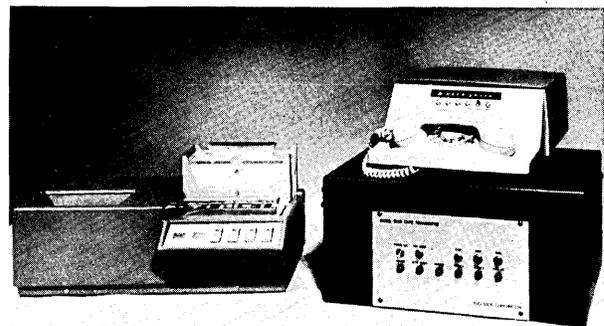
In addition to our line of converters, Digi-Data Corporation manufactures card and paper tape Data-Phone® transmission units such as the Model 2120 Magnetic Tape Receiver and the 2020 Card Transmitter shown here.
