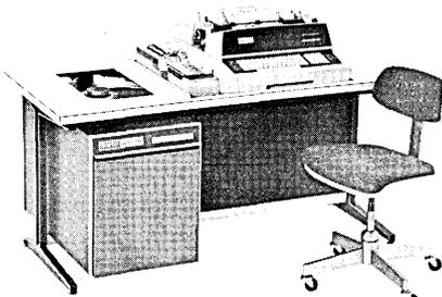
— To the left of the Input-Output Station is a horizontal tape transport. The electronic processor, below the transport, is the control center for the complete 5610 system
