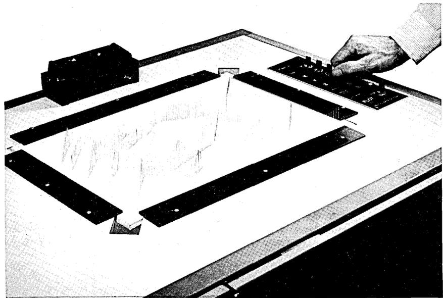
The 11 x 17 Plotter will plot (with correct buffer electronics) 3-D data from electronic processors, magnetic and paper tape, and punched cards. Accepted by the basic unit are 7-bit code; 6 bits (representing positive and negative increments of X, Y and Z); and 7th bit (indicating a plotting point). Plotting is limited only by the size of the X-Y positioning mechanism. The surface of the plotting board can be annotated before/after plot is made, with ink or pencil. Full
