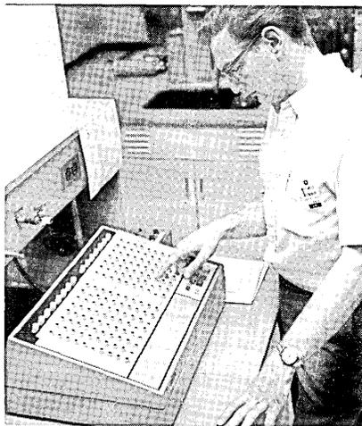
puter what technique to follow. The IBM 1800 computer, located adjacent to the control lab, is programmed to run the sample through a testing instrument and interpret its data. Results are printed on an output typewriter and furnished manufacturing personnel.
