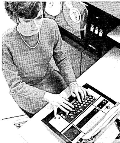
The new devices prepare computer-ready half-inch magnetic tape compatible with all Honeywell Series 200 computer systems, from the new small-scale H-110 (see New Products, Digital) through the large-scale H-8200, and with most computer systems of other manufacturers.
