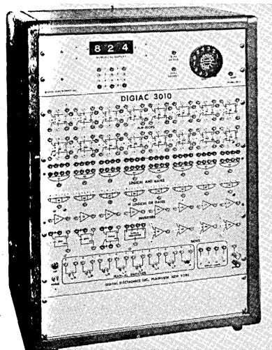
A telephone dial and numerical display panel combine to serve as an input-output device which simulates entering and retrieving data from a computer. Designed for continual use, the 3010DD uses solid-state components mounted on individual printed circuit boards. It also contains built-in short-circuit protection. A removable rear panel provides access to all components for instruction in computer maintenance and servicing. (For more information, designate #41 on the Reader Service Card.)
