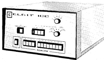
programmable for optimizing speed of real time operations, has a typical add time of 6 usec for a full twelve bit word, and can operate with up to 256 different I/O devices. (For more information, designate #44 on the Reader Service Card.)
