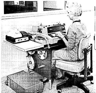
Autofax offers two-way communication with a centralized data processing location. Data signals from typewriters, adding machines, punched tape, magnetic tape, punched cards, etc. are converted into tones. These are transmitted over existing telephone lines at 200 words per minute. Autofax system equipment has built-in error control circuits for correct data transmission.
