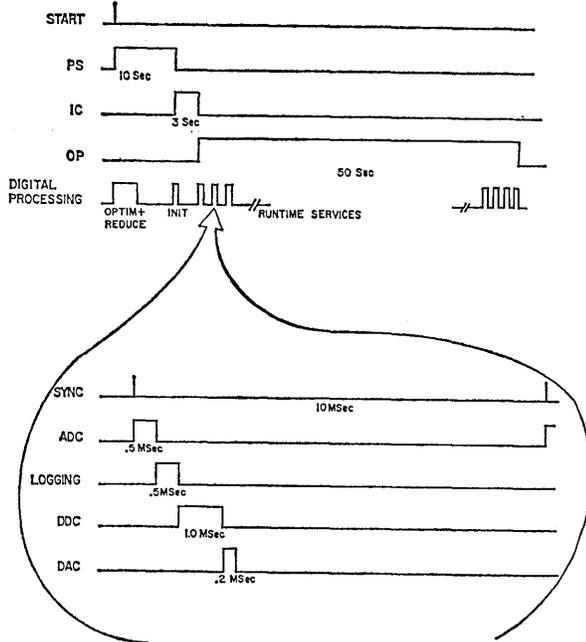
As usual, the speed of the hybrid model was limited by the speed of the run-time digital program. While the execution time of RUNTIME is approximately 2.5 milliseconds, only one fourth of the 10 millisecond cycle time, the analog speed, or time scale, can be conveniently changed only in multiples of ten. Also, additional run-time services were planned which would have increased the execution time of RUNTIME. For these reasons, no attempts were made to increase the speed of the hybrid model.
