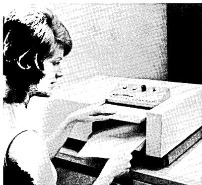
and the copy which is scanned by line is fed by ordinary telephone lines to a central recognition unit capable of converting the data to punch paper, magnetic tape or punch cards. Since this scanner is located on the user's premises, original documents never have to leave the client. A single unit, as pictured above, can scan with 100% accuracy and convert to computer language the equivalent amount of work done by 12 key punch operators.
