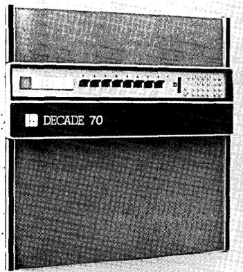
The basic machine is available with a 4,000 word memory and is internally field expandable to 16,000 words. Mr. Linebarger says that the Decade 70/2 is a 16 bit machine yet is competitive with 12 bit units. Memory cycle time is 900 nanoseconds.
