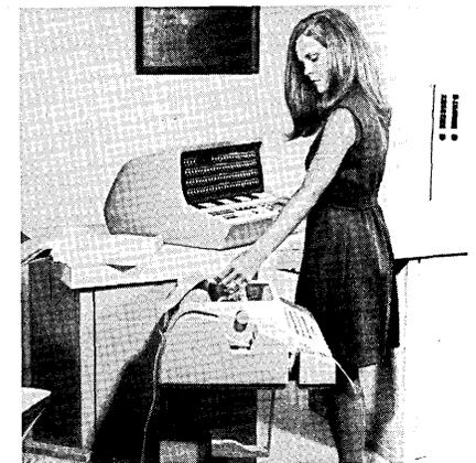
The basic DC-6024 processing unit includes five 24-bit general purpose registers, three of which also may be used as index registers; 4K-word memory (12,288 bytes); hardware multiply/divide/square root; and four true levels of priority
