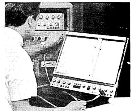
Listed features include true differential input, common mode rejection, high speed, time base (Model 530T) and computer reference optional capability. Model 530 is said to incorporate design and op-
