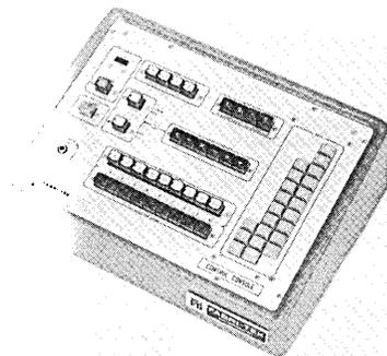
Two control keys permit the instructor to perform mathematical operations without a stored program and to give an effective demonstration of binary arithmetic. They also simplify setting up either manual or external I/O operations, reduce initial programming time requirements and allow more effec-
