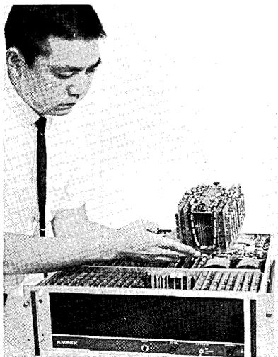
An engineer demonstrates how the core stack can be removed easily from the Model RGX core memory.
