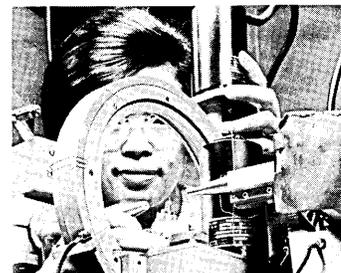
The front cover shows a laboratory technician positioning a tiny crystal of food on an X-ray diffractometer for analysis. The task is to isolate and identify each component contributing to a food's particular flavor and aroma. The instruments used in the analysis are controlled by a computer. For more information, see page 57.
