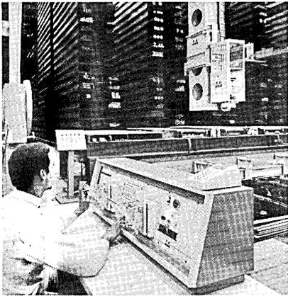
ized materials handling system controls the cranes by feeding punched cards into a central computer console as shown in the picture above.
