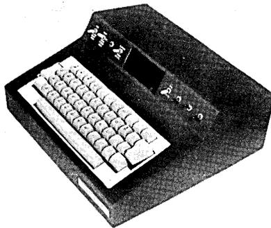
stored. The stored data is transferred to magnetic tape or transmitted directly to a computer on demand. Each of up to 32 keyboards can simultaneously perform data entry, verification, search and error correction.
