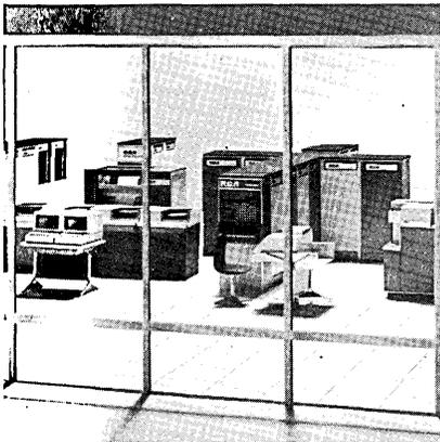
— RCA Spectra 70/60 system. The processor, center rear, is shaped like a large plus sign.
