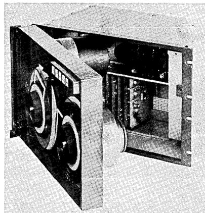
— Interior view of BI 830 showing vibration free front casting and heavy duty printed circuit motors
