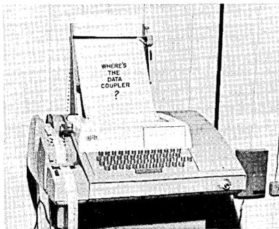
The terminal, suited to a wide range of applications such as time sharing, terminal to terminal communications and computer access, transmits and receives at 100 words per minute. A fully filtered transmitter and receiver data set rejects harmonic and spurious signals assuring error free transmission.
