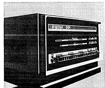
Initially the PDP-11 will be offered in two models: a special purpose controller, the PDP-11/10, equipped with central processor, 1024 words of read-only memory, and 128 words of standard memory; and the PDP-11/20, a general purpose computer with central processor, 4096 words of standard core memory expandable to 32,768 words, a programmer's control panel, and Teletype. (For more information, circle #43 on the Reader Service Card.)
