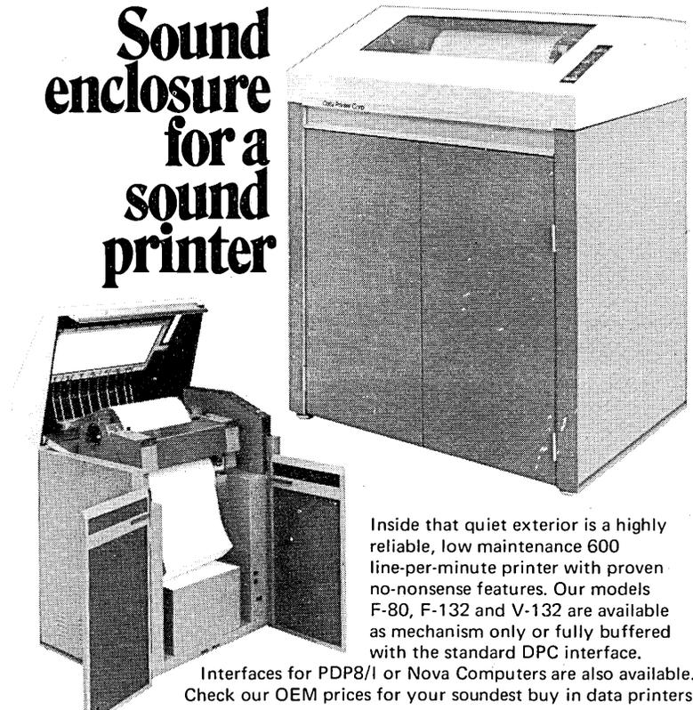
Inside that quiet exterior is a highly reliable, low maintenance 600 line-per-minute printer with proven no-nonsense features. Our models F-80, F-132 and V-132 are available as mechanism only or fully buffered with the standard DPC interface.
