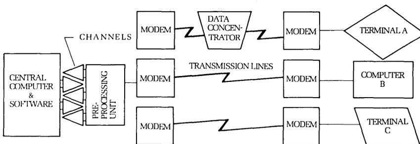
Figure 1. Typical Data Communications Network
