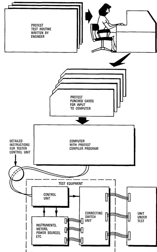
Figure 1 - A block diagram of PROTEST equipment.
