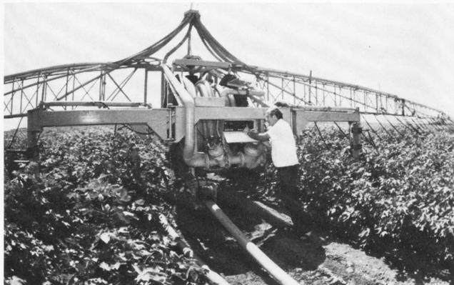
Only one man is needed to irrigate 350 acres a week using this self-propelled irrigating sprinkler system developed in Israel. The only human attention it needs is adjustments to its microprocessor which monitors speed and controls water output. The computer shuts off the machine if any malfunction occurs.
