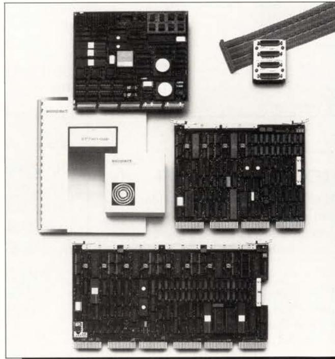
*Simpact's BSC communication protocol interfaces for the VAXBI bus, Q-bus and UNIBUS.*
