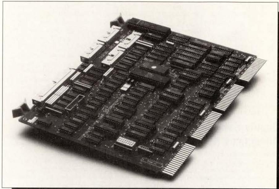
*DILOG's new DU236 UNIBUS SMD controller offers configuration and throughput enhancements.*
