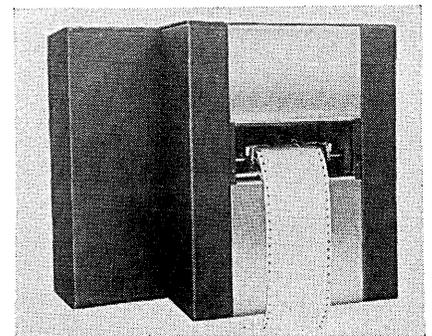
POTTER INSTRUMENT Co., INC., Sunnyside Blvd., Plainview, L. I., N. Y., has announced a new high-speed alphanumeric digital printer, Model 3260, that can print more than 400 digits or characters per second, and may be connected to most data producing sources with little modification.
