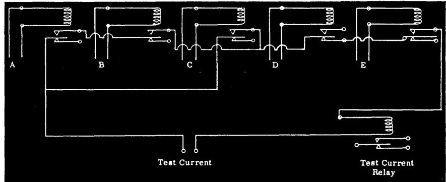
Figure 4. Circuit diagram to illustrate detection of logical relationship,  $(A \cdot B + C) (E - D)$ .
