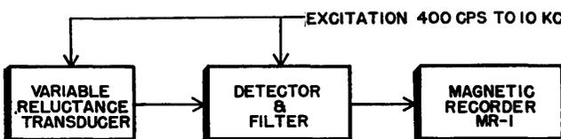
Fig. 6. Typical variable reluctance transducer circuit.
