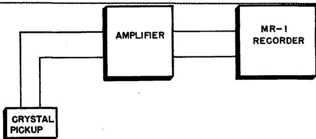
Fig. 5. Typical connection of piezoelectric transducer through amplifier.
