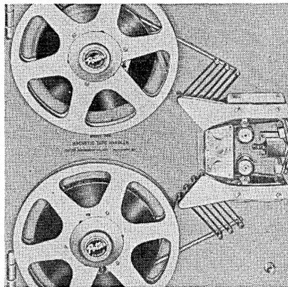
POTTER INSTRUMENT Co., INC., Sunnyside Blvd., Plainview, L. I., N. Y., has announced a completely-transistorized digital magnetic tape handler, Model 906. Both high and low tape speeds are available in the new unit in ranges of 4 speeds forward and reverse up to 150"/sec. Rewind or search tape speeds are 400"/sec.
