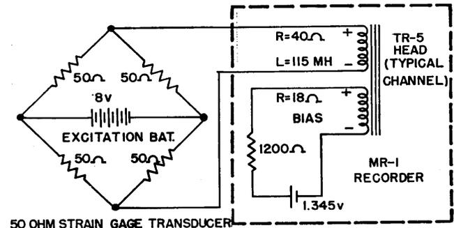
Fig. 4. Typical strain gage circuit.
