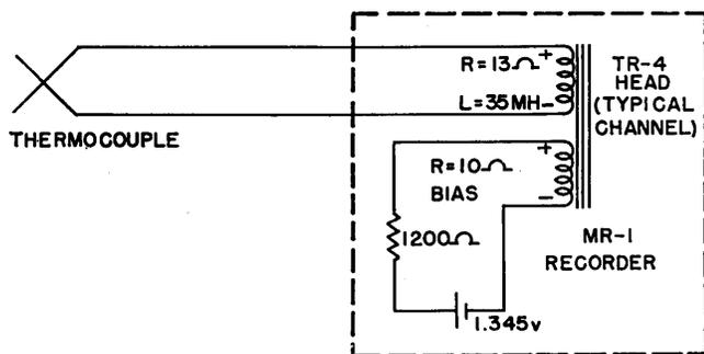
Fig. 3. Typical thermocouple circuit.
