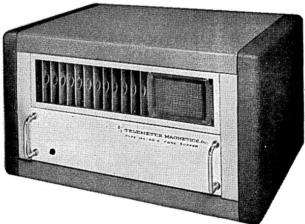
**SPECIFICATIONS:** Number of characters: 144; Number of bits/characters: 8\*, loaded or unloaded simultaneously; Loading or Unloading Speed: 14 µ sec/character; Solid state components only. Signal Amplitudes: Input: ZERO-5 Vdc, ONE+5 Vdc, Output: Pulse: ZERO-5V, one +5v. Load Sync: +10v, Unload Sync: +10v. Power: 1 amp at 115v, 60 cps.
