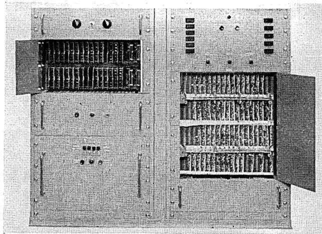
*Designed for the Florida Automatic Computer, FLAC high-speed output buffer system will accept information at rates from 6 to 8 kc, make it available to any 1 of 6 punches at rate of 60 characters/sec.*
