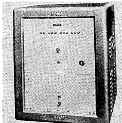
EPSCO, INC., 588 Commonwealth Ave., Boston 15, Mass., announces their Model K Dattrac—a high-speed voltage-to-digital converter that makes possible high-speed, on-line entry into digital computers. A single connection to the cable (furnished with equipment) links the unit to the digital computer input register.
