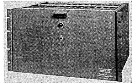
EpSCO, Inc., Components Div., 108 Cummington St., Boston 15, Mass., has developed and is now marketing a magnetic core buffer storage unit, Model CB-602/1000, that has a total storage capacity of 1000 bits of information. Construction is modular; assemblies of lesser storage capacity are available.
