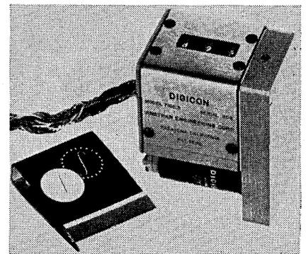
or ground test units and provides a visual as well as electrical readout with either potentiometers or contacts opposite each number wheel. It provides continuous voltage outputs from each number wheel proportional to the number indicated in the counter window.
