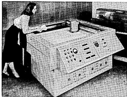
freedom in presenting output data in graphic form. Accepting information from punched paper tape, punched cards or magnetic tape, the unit oper-
