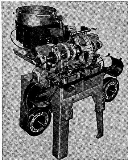
feature of the tip application is the prevention of cold solder problems by eliminating any movement of components during dipping cycle. The tip permits bridging or offsetting of components to improve air circulation and to eliminate temperature influence. Design of the tip promotes solder-wicking and uniform solder deposit and also protects fine semiconductor leads from heat and assembly damage. For information write AMP INCORPORATED, Harrisburg 34, Penna. Or use reader card.
