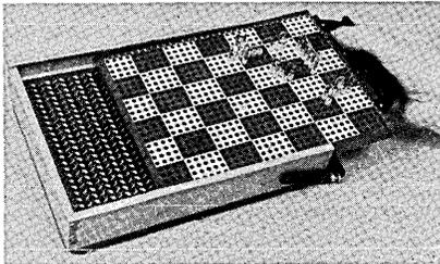
ated which permitted the systems to be mounted edgewise—turned on their side and assembled "building block" fashion resulting in a minimum of space being required. In this application, the programming systems are employed as a pluggable chassis. The removable patchcords serve as the chassis and the patchcord tips mating with the contact springs function as a
