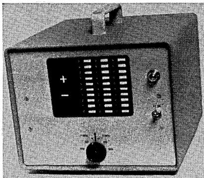
ures voltages to a full-scale accuracy of better than one-half of one per-cent. It operates from a 117-volt AC source (20 watts) and consists of transistorized computer elements including a precision digital-to-analog converter, comparator, logic and a reference power supply, which is held to an accuracy of better than one-tenth of one percent. For information write RANSOM RESEARCH, 323 W. 7th St., San Pedro, Calif. Or use reader service card.
