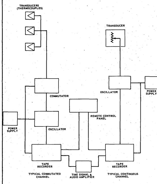
Figure 1: Block Diagram of Airborne Data Accumulation System
