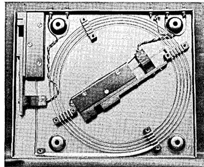
10 in. x 3/8 in., weight - approximately one pound, attenuation - 50 db approximately, signal to noise ratio - greater than 20:1, and delay adjustment range - 4 microseconds. For information write FERRANTI ELECTRIC, INC., Electronics Div., 95 Madison Ave., Hempstead, L. I., N. Y.
