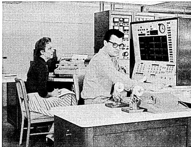
*Miss Loretta Kassel and William Snow, programmers, check a program of instructions at the console of GEORGE, a computer recently installed at Argonne National Laboratory, Lemont, Ill. Snow is feeding punched tape through a high speed reader while Miss Kassel checks data from an electric typewriter, an output method used to obtain program results at a slower speed.*
