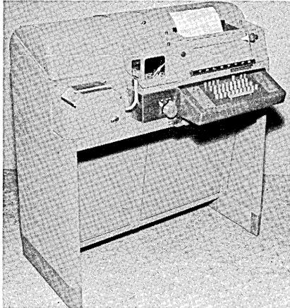
It incorporates combinations of the following model 28 basic mechanisms in a single, compact console: keyboard base, page printer, perforator, tape transmitter, motor unit, and electrical service unit. For information write TELETYPE CORP., 4100 Fullerton Ave., Chicago 39, Illinois.
