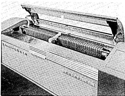
(500-million in the Datatron 220), through the use of the new Datafile multiple magnetic tape units. One Datafile "bin" can store 20-million characters. Up to 10 units can be integrated into one computer system. Conventional tape reels are replaced in the
