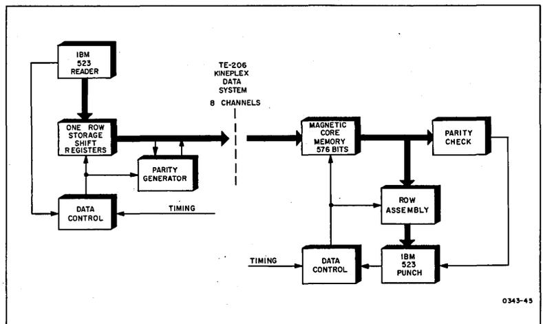
Fig. 5: Kinecard converter simplified block diagram
