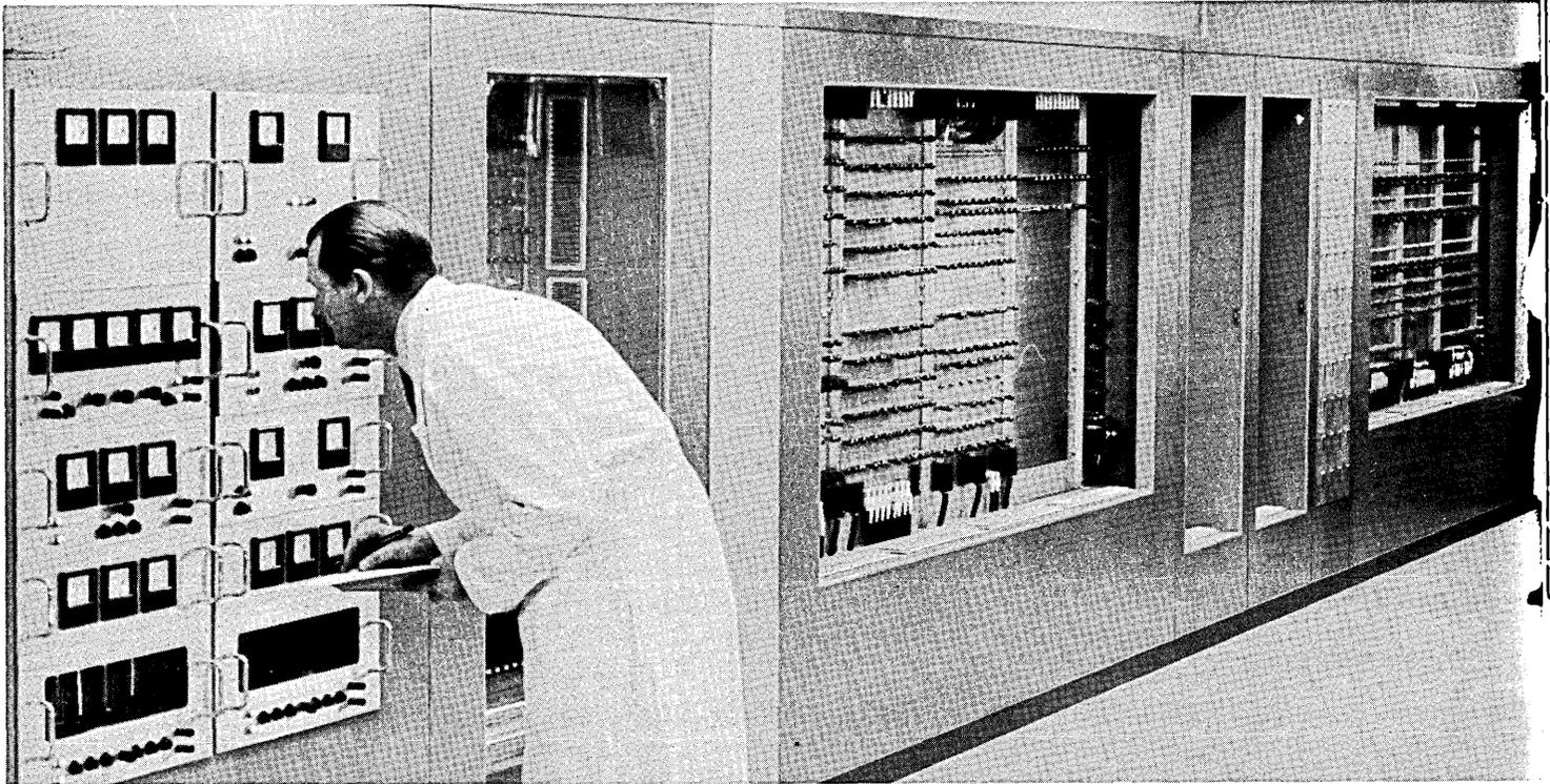
*Left to right, SARA's power supply, drum, control, memory and arithmetic units, control desk relays and storage buffer unit.*
