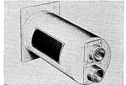
less than half the space of conventional designs. The converter is made for both ac and dc power supplies and has a wide full scale range adjustment. Full scale input frequency is adjustable from 300 to 900 cps with a minimum frequency of 10 cps. Output voltage is 0-5 v dc into a 500,000 ohm load; 0-100 mv dc into a 10,000 ohm load; or 0-50 mv dc into a 5,000 ohm load. For information write FISCHER AND PORTER CO., 752 Jacksonville Rd., Hatboro Penna. or use card.
