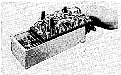
system, weighs 3¼ lbs. and has been miniaturized to conserve space. Removable, pre-patched boards make complete circuitry reprogramming possible in a matter of seconds. The unit itself is constructed of aluminum alloy and will withstand shock and vibration, according to the manufacturer. Seating of patchcord pins are also designed for shock resistance. For versatility of circuit combinations, the
