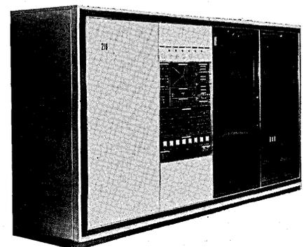
Laboratory at Langley Field, Va. Model 210 will be capable of sampling wind tunnel information at the rate of 3,000 signals per second. The information from transducers within the tunnel being served will be fed to the system and recorded as tem-
