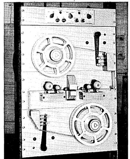
characters per second, with less than 5 milliseconds start or stop time. At 300 characters per second it stops in the space following the stop character. For 750 character per second operation, a two character stop space is recommended. All standard 5, 6, 7 or 8 level tapes (plus sprocket hole) are handled and 11/16 in., 7/8 in. or 1 in. wide tapes can be used interchangeably. Other characteristics include complete remote control of forward,
