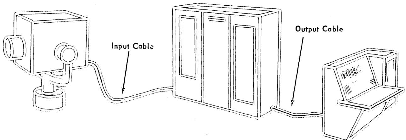
**Sensory System:** Input camera, with aiming servos, which allow Perceptron to center or track moving objects.
