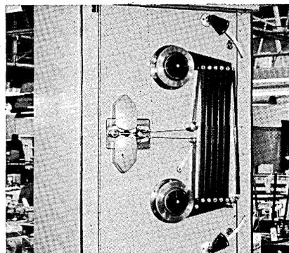
The continuous loop adapter permits study of transients in rocket engine tests, wave analyses by means of time compression, and similar operations. The adapter can be attached with a screwdriver. Its upper and lower arms are adjustable to accommodate loop lengths from two to 26 ft. Three models are available for standard instrumentation tape widths of 1/4-, 1/2- or one-inch. For information write Consolidated Electrodynamics Corp., 300 N. Sierra Madre Villa, Pasadena, Calif.
