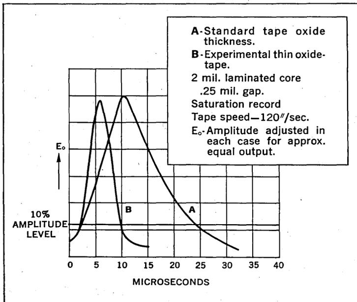
Pulse width comparison—standard and thin oxide tape.
