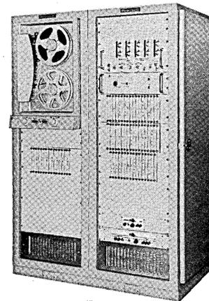
function — digital systems can be assembled to multiplex and digitize data at rates up to 15,000 samples per second within an accuracy of 0.05 per cent, according to the manufacturer. Using the modules in various arrangements, it was explained, operators can engineer digital systems to
