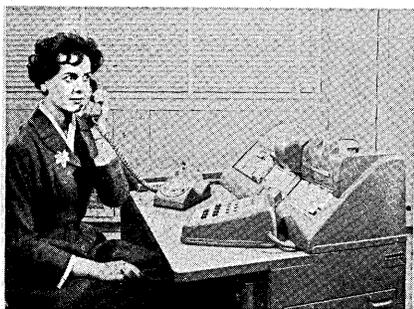
lar toll telephone calls — have been announced. The 7701 magnetic tape transmission terminal sends business and scientific data at the rate of 150 characters or thirty words a second. The data transceiver equipped with a dial-up telephone feature, can trans-
