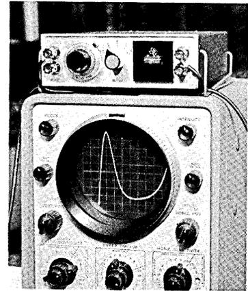
rather than just a portion of that curve. Through the use of an external decade box shunted across the horizontal terminals, it is practical to read the actual negative resistance of the tunnel diode at any point on the curve. For information write TEXAS INSTRUMENTS, 3609 Buffalo Speedway, Houston 6, Texas, or use card.
