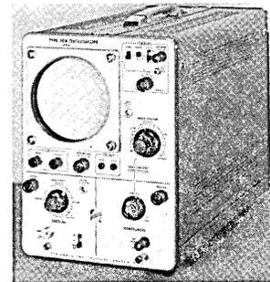
put stage electronically regulated, calibrated steps to 20 v/cm, adjustable between 12 steps and to over 50 v/cm uncalibrated, and constant input impedance (for easy probe use) at all sensitivities. Other features include: functional panel layout, 8 x 10 cm viewing area, 18 calibrated sweep rates, electronically-regulated power supplies, and extremely adaptable trigger facilities. For information write TEKTRONIX, INC., P.O. Box 831, Portland 7, Oregon, or use card.
