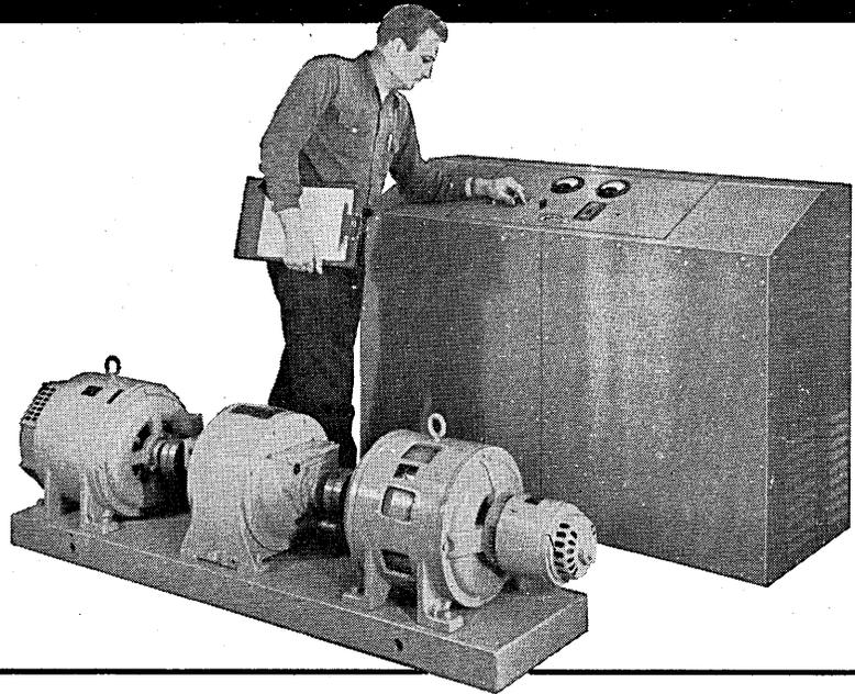
**The modern way** to boost electronic power-system reliability is also the best way to cut cost, size, heat-loss, and complexity...by interposing a precisely-regulated motor-alternator set as a buffer-regulator between your DC power supplies and the power line. Typical Savings: 50-90%.
