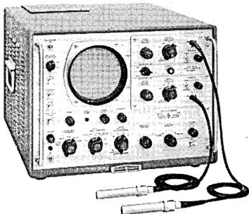
a single package, conceived to permit operation similar to a conventional oscilloscope. Model 185A has a rise time of less than 0.7 mus. Its full 10 centimeter vertical display and high
