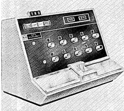
by computers to process such items as payroll, work-in-process inventory, costs and scheduling operations. The 180 Data Collector automatically assembles into a punched paper tape variable data (such as job-lot number and amount produced), identification data from pre-punched IBM cards (such as employee number & item number), fixed data (such as department number and Data Collector number), and time from an internal clock (to the nearest 0.01 hour). The
