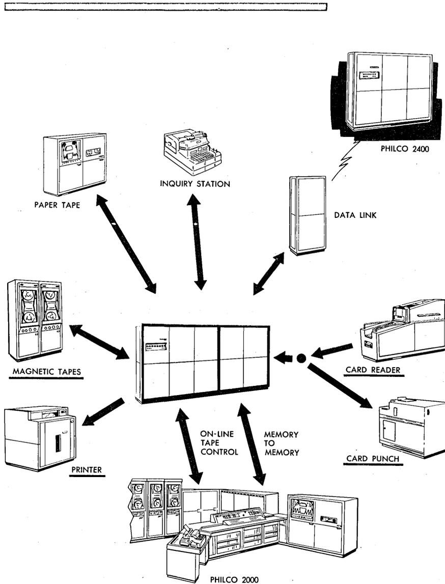
Expanded Philco 2400 for Data Traffic Control. Underlined captions comprise basic system: tapes, card reader, card punch, printer.
