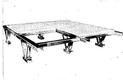
designed to support a live load of 250 lbs. per square foot, and a point load of 1000 lbs. Steel stringers are bolted to a new kind of adjustable jack designed in a triangular shape. Deflection is claimed to be minimized under even the heaviest loads, STRATO-FLOOR, INC., 795 East 152nd St., Cleveland 10, Ohio. For information:
