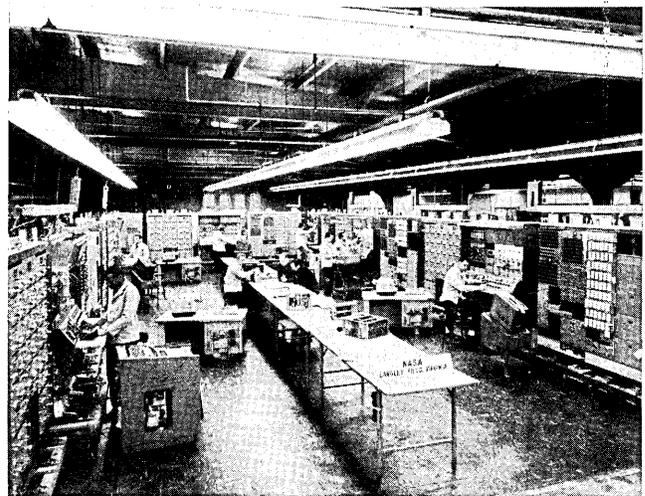
The world's largest general purpose analog computer, designed and built for the National Aeronautics and Space Administration, is seen undergoing final inspection and check-out at Electronics Associates, Inc. West Long Branch, N.J. All units of the computer were installed at NASA's Langley Field, Va., research center this spring. It occupies more than 1,800 sq. ft of floor space and comprises five separate PACE 231R computer consoles.
