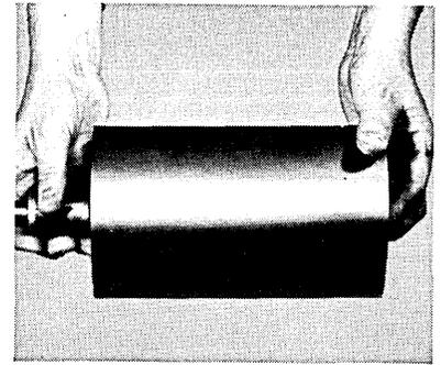
**JANUARY 1961—9200-word drum developed for Univac Solid-State 80/90 central processors**
