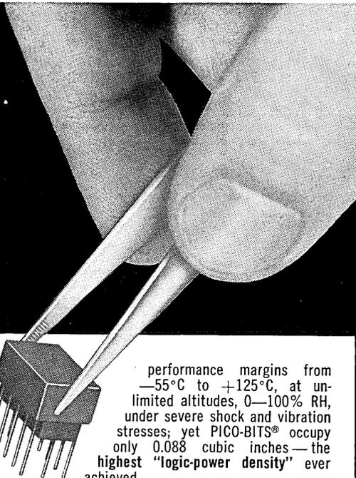
PICO-BITS® are micro-micro packages of our time-and-space-proven magnetic logic circuitry. A single PICO-BIT® can perform any basic logical function: AND, OR, INHIBIT, (AND NOT), BRANCH, STORE, TRANSFER, DRIVE, BINARY COUNT, or COMPLEMENT — greatly simplifying circuitry, minimizing semiconductors.
