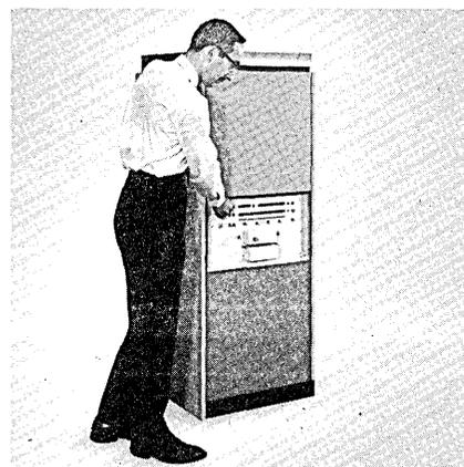
The 910 is the first random access, buffered input/output digital computer to be priced below \$90,000. Although designed primarily for systems use, its high speed, working flexibility, and excellent performance allow it to be used as an extremely low cost general purpose machine. The 910 operates directly, without special coupling, with all types of input/output devices, including magnetic tape units, A-D converters, automatic typewriters and line printers.
