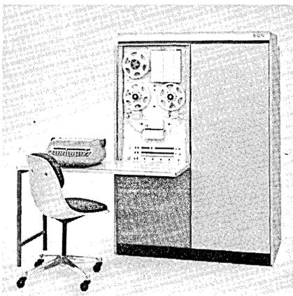
The 920 is an extremely fast, general purpose computer for scientific use. Its command structure includes built-in Floating Point and Multi-Precision instructions. In speed, characteristics, and working flexibility, it surpasses larger, more costly first generation solid state machines. When carefully compared on all of its operating parameters, the 920 clearly offers more general purpose scientific computing-per-dollar than currently available machines.
