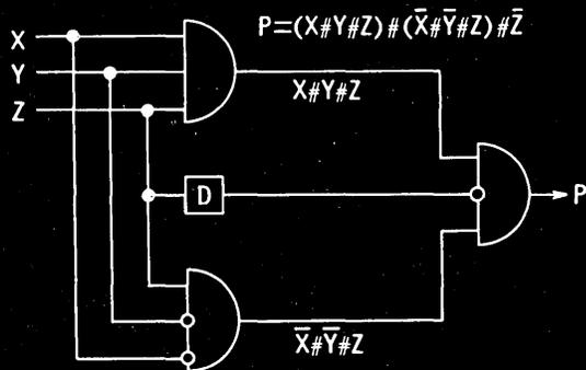
The fundamental theorem of majority-decision logic, a typical product of Univac's Mathematics and Logic Research Department, has practical as well as theoretical interest. The even-parity checker derived above from the fundamental theorem can be freed to determine the parity of  $3^n$  bits in  $2n$  logic levels using only  $\frac{3}{2}(3^n - 1)$  three-input majority gates.
