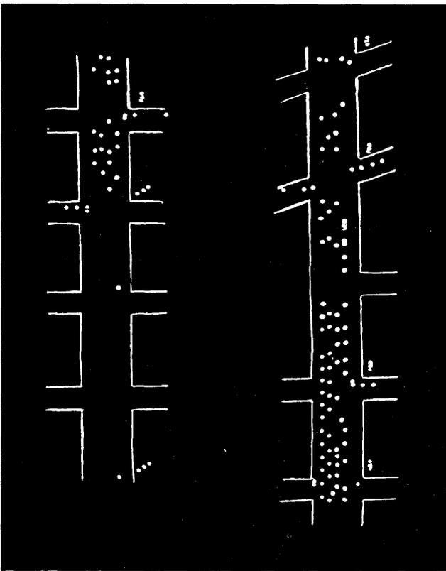
Single frame of motion picture produced from oscillograph. The course is photographed in two segments, beginning at lower right, ending at upper right. Traffic lights are shown as a bar of three lights: vertical configuration indicates green for 13th St. traffic, horizontal red, and diagonal amber. Single dots represent cars, double dots small trucks, and triple dots large trucks.
