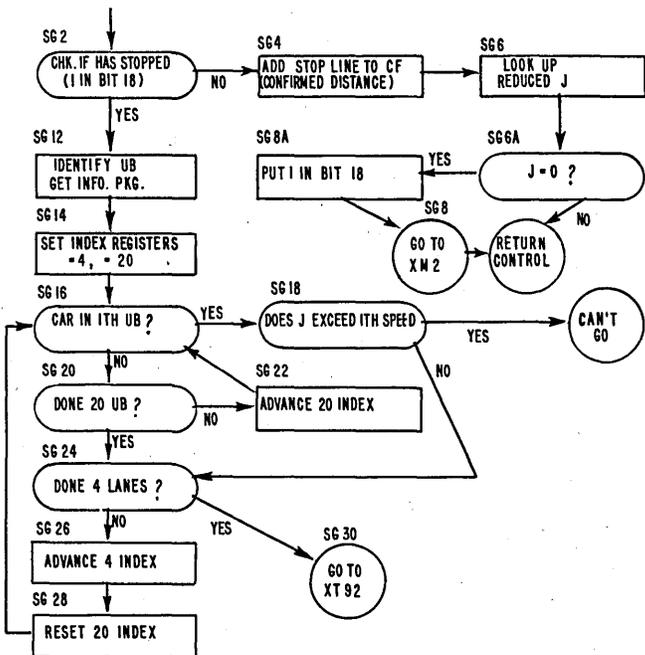
Flow chart of Stop Sign Routine. Before the car can proceed across the intersection, 20 approaching Unit Blocks are checked in each of the four lanes. If another car is present or moving, the car cannot proceed. Should an opposing car be farther away but moving at a critical speed, the stopped car cannot proceed.
