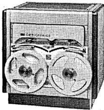
omni-data photoelectric reader with reeler, Model PTR-70250A. Reads any type of tape—punched or recorded, opaque or transparent—with chopped reflected light. Offers start-and-stop asynchronous action up to 60 steps per second. Unidirectional, with rewind and no tape breakage.
