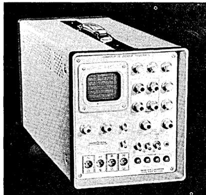
tions as analog to digital conversion, recording fast wave forms, plotting of digital data, statistical distribution of analog and events and function generation. MNEMOTRON CORP., 45 S. Mail St., Pearl River, N. Y. For information:
