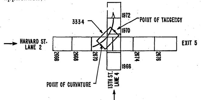
When making a simple turn, the car progresses through Unit Blocks 2666-2668-2670-3334-1970-1972. All information for making the turn is contained in UB 2670, such as if the car will turn, direction of turn, which lane car will enter after turning, and exit if car will not turn.
